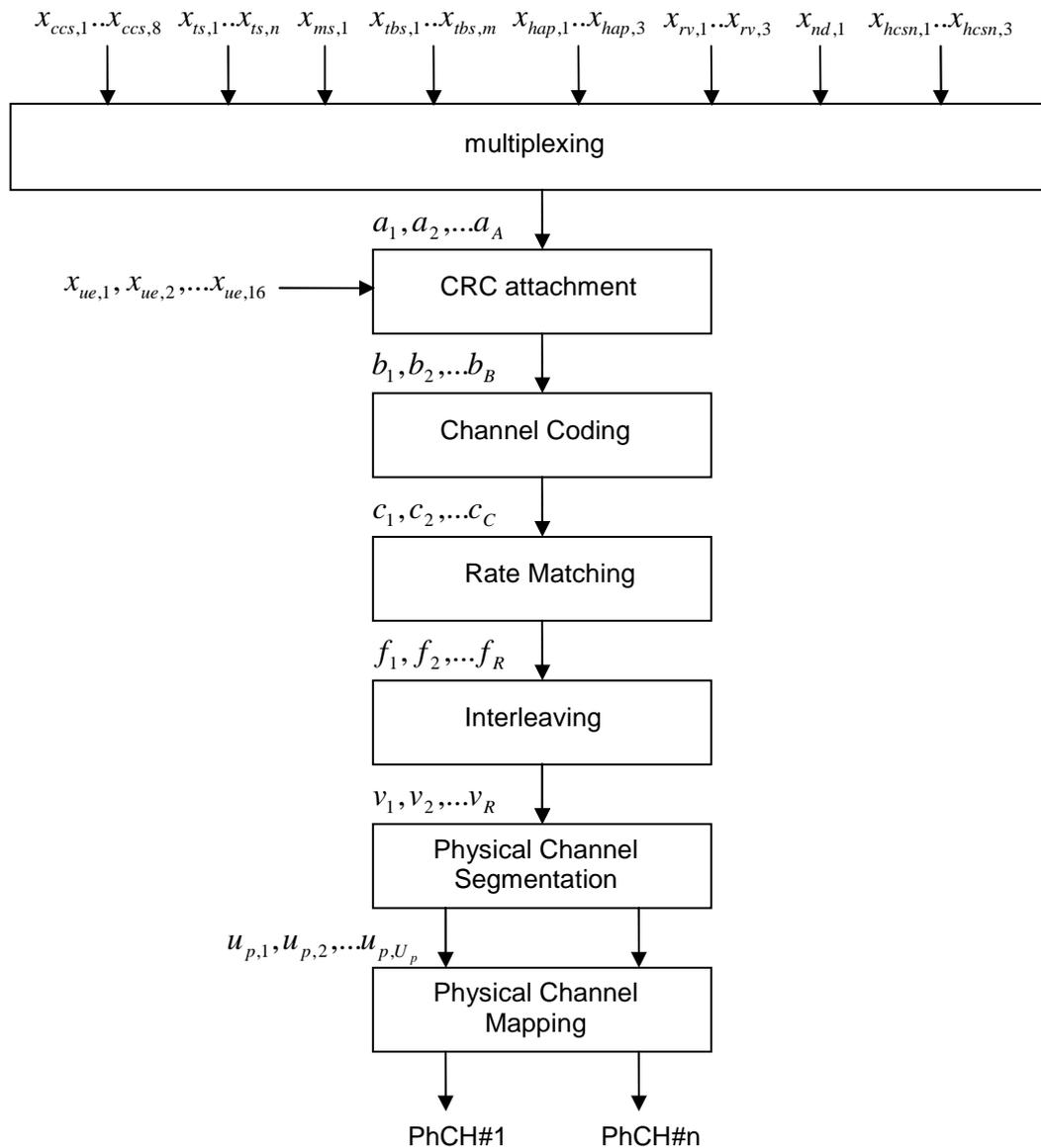
Figure 18c Coding and Multiplexing for HS-SCCH
