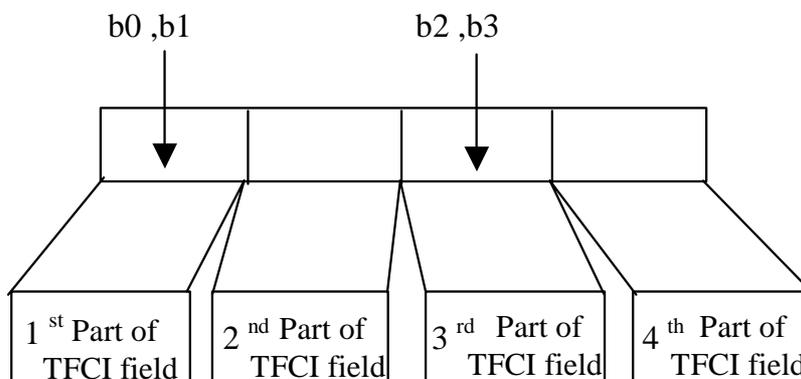
**Figure 11: Mapping of TFCI code word bits to TFCI position in 1.28 Mcps TDD option, when  $N_{\text{TFCI code word}} = 4$**
