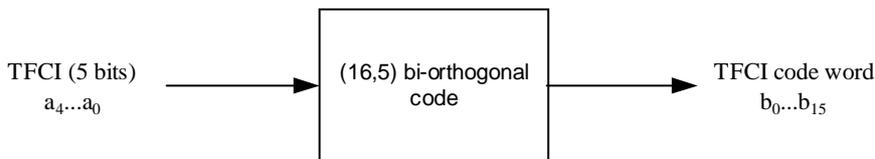
Figure 8: Channel coding of short length TFCI bits
