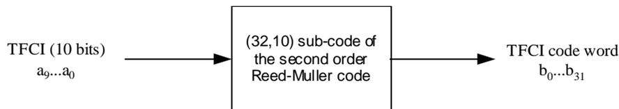
**Figure 7: Channel coding of the TFCI bits**
