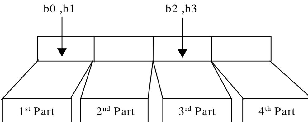
**Figure 10: Mapping of TFCI word bits to TFCI position in 1.28 Mcps TDD option, when  $N_{TFCI}=4$**
