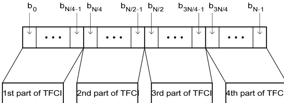
**Figure 9: Mapping of TFCI word bits to TFCI position in 1.28 Mcps TDD option, where  $N = N_{TFCI}$ .**
