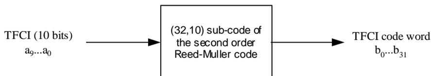
**Figure 6: Channel coding of TFCI information bits**
