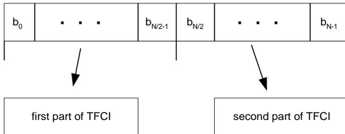
**Figure 8: Mapping of TFCI word bits to timeslot**
