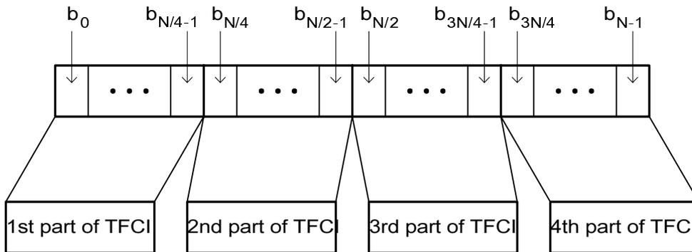
**Figure 13: Mapping of TFCI code word bits to timeslot in 1.28 Mcps TDD option, where  $N = N_{TFCI}$ .**
