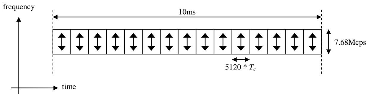
Figure 6.1.1: The 7.68Mcps TDD option frame structure
