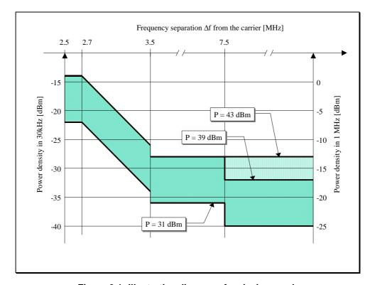
Figure 9.1: Illustrative diagram of emission mask
