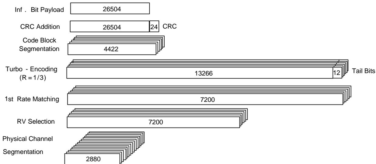
**Figure A.26: Coding rate for Fixed Reference Channel H-Set 11 Primary Transport Block**
