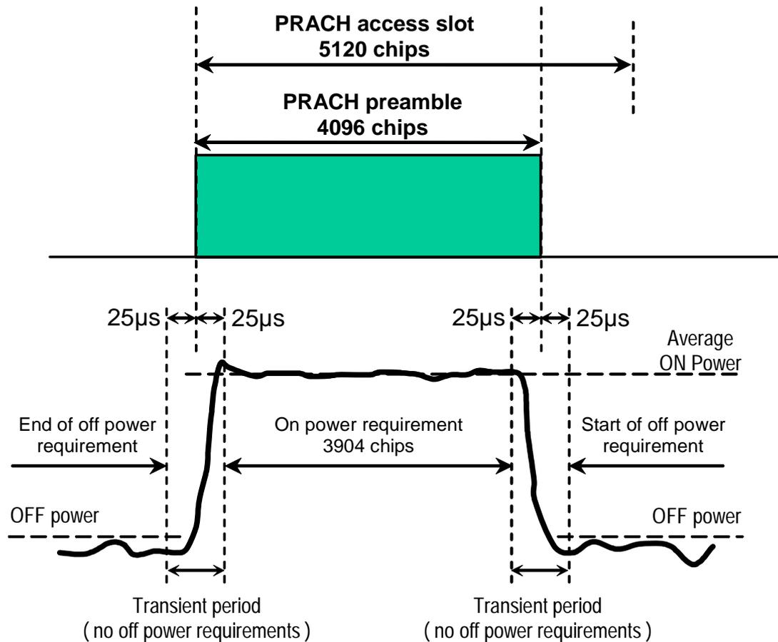
Figure 6.2: Transmit ON/OFF template for PRACH preambles
