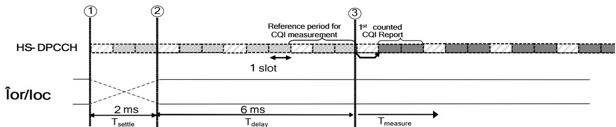
Figure 9.2 Timing relation between HS-DPCCH, DPCCH/DPDCH and  $\hat{I}_{or}/I_{oc}$  ramping. The measurement equipment starts ramping the  $\hat{I}_{or}/I_{oc}$  at point 1. The  $\hat{I}_{or}/I_{oc}$  should be settled to its nominal value at point 2. The first CQI report that is counted in the statistics of the requirement is transmitted in the uplink at point 3.
