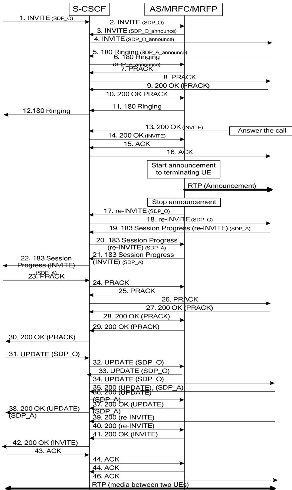
**Figure A.14: Announcement provided to the terminating UE when the called user answers the call and prior to establishing media stream between end users**
