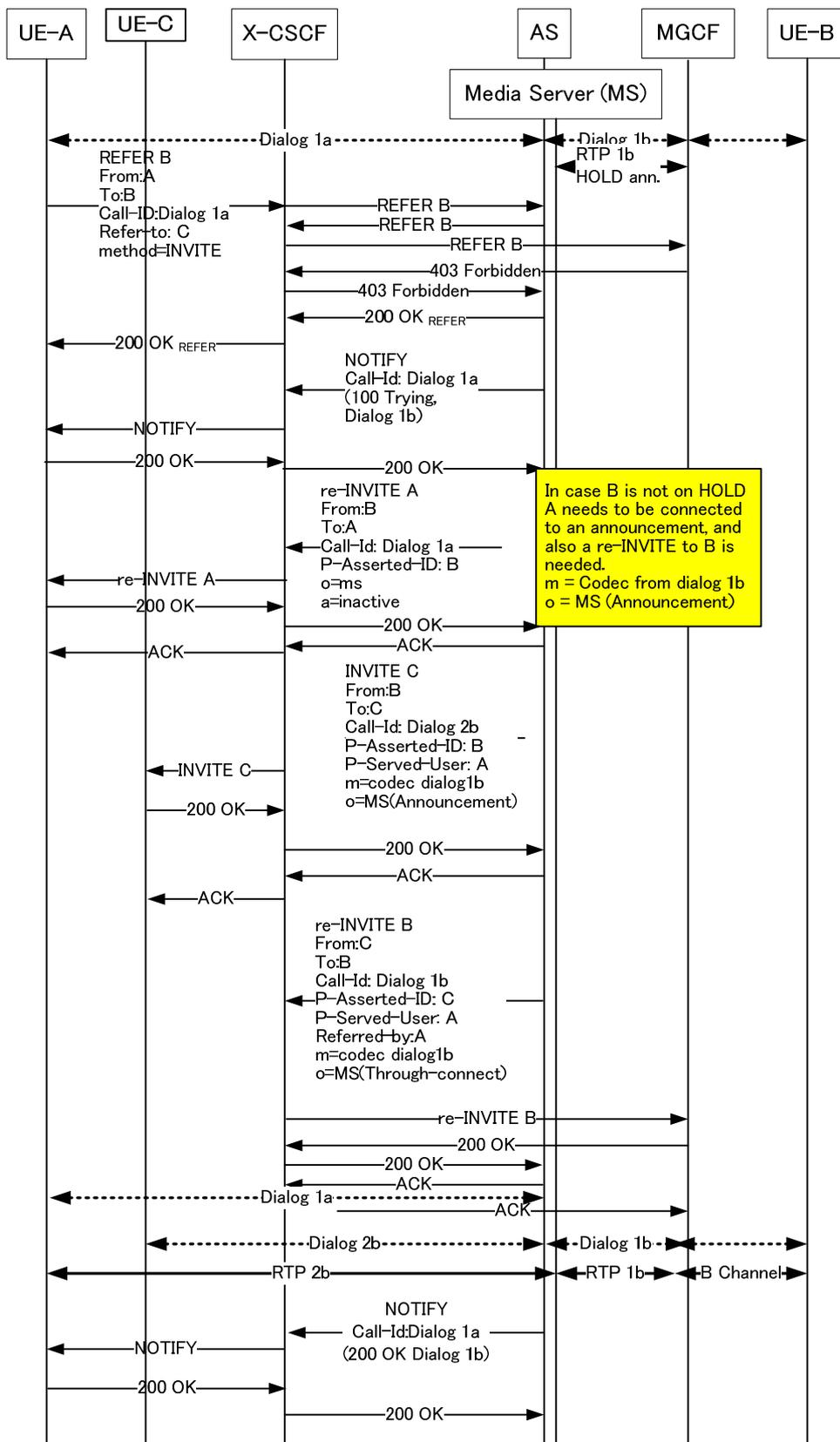
Figure E.1: Example flow for REFER interworking with REFER sent inside a dialog with usage of a media server
