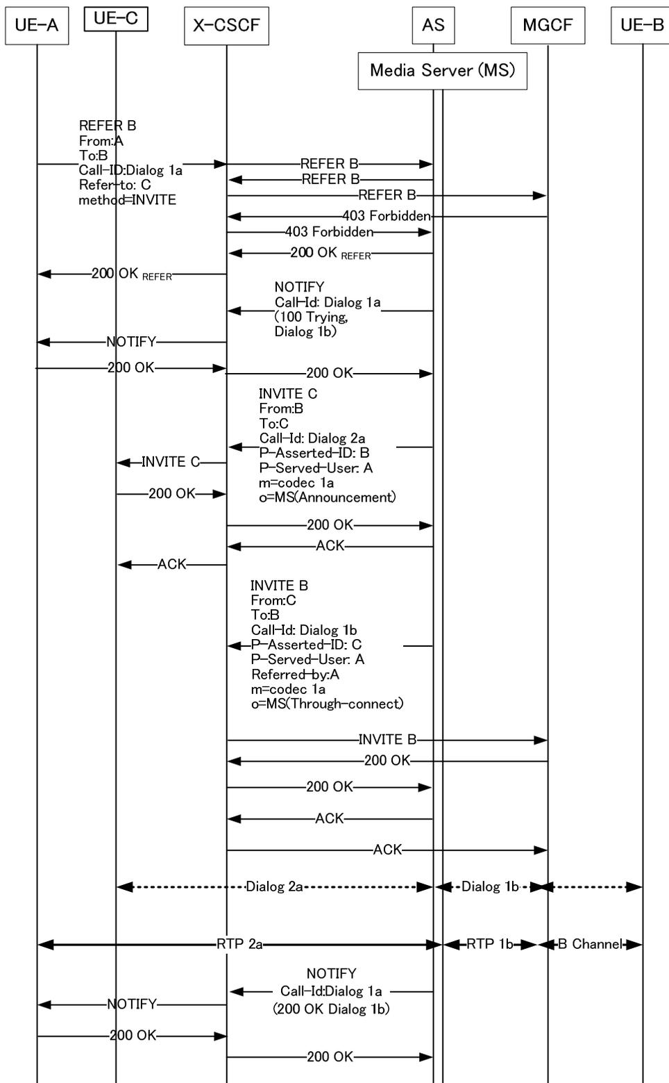
Figure E.2: Example flow for REFER interworking with REFER sent outside a dialog with usage of a media server
