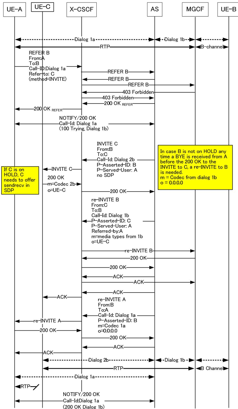
Figure E.5: Example flow for REFER interworking with REFER sent inside a dialog without usage of a media server
