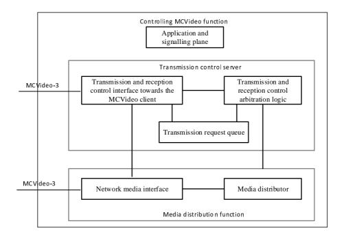
NOTE: The real internal structure of the MCVideo server is implementation specific but a possible internal structure is shown to illustrate the procedures.
