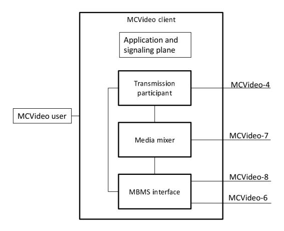
NOTE: The real internal structure of the MCVideo client is implementation specific but a possible internal structure is shown to illustrate the logic and the procedures.
