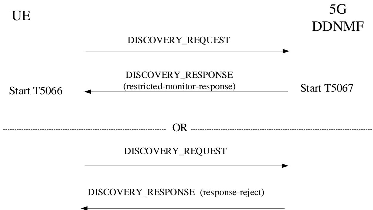
**Figure 6.2.5.2.1: Monitor request procedure for restricted 5G ProSe direct discovery model A**
