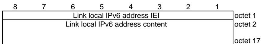
**Figure 11.3.7.1: Link local IPv6 address information element**
