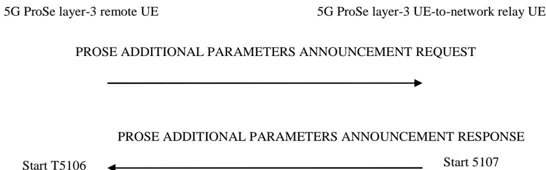
**Figure 8.2.8.2.1: 5G ProSe additional parameters announcement procedure**
