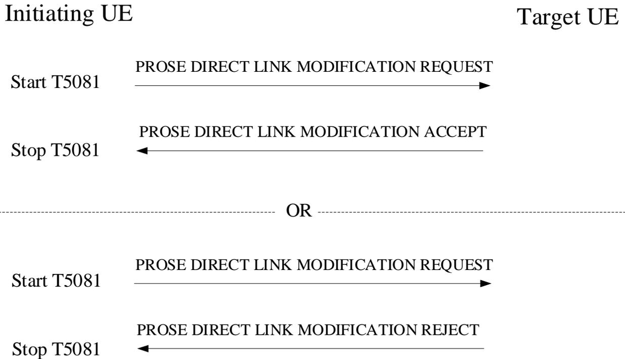
Figure 7.2.3.2.1: 5G ProSe direct link modification procedure
