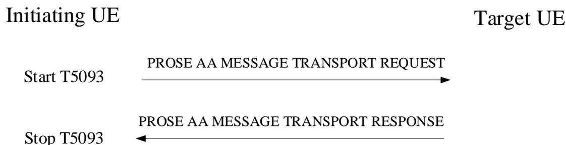
Figure 8.2.9.2.1: 5G ProSe AA message reliable transport procedure
