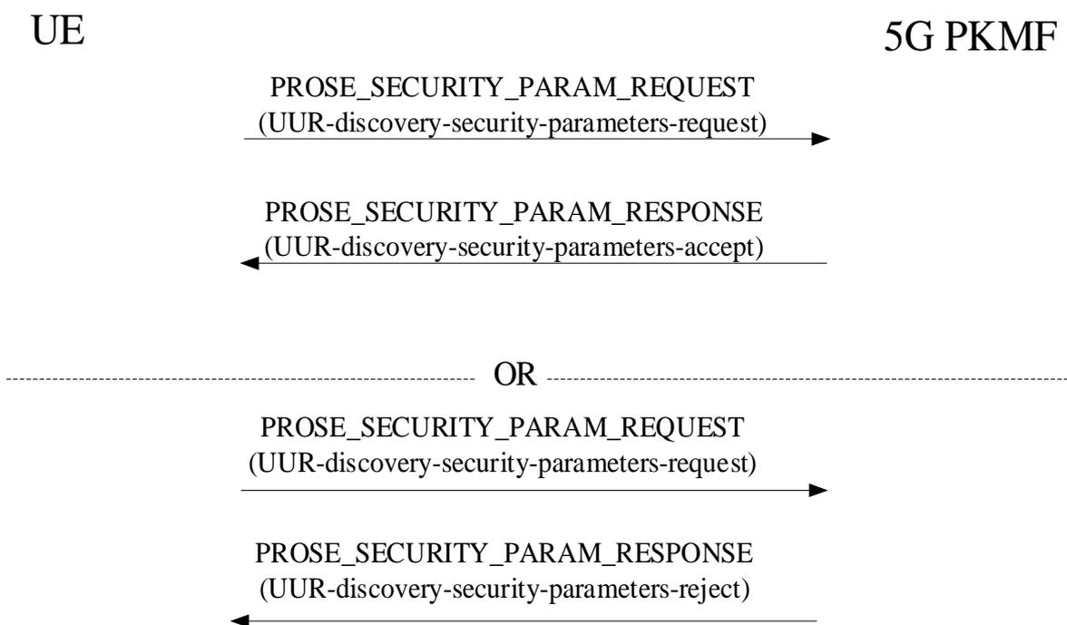
**Figure 8a.2.12.2.2.1: 5G ProSe UE-to-UE relay discovery security material request procedure**
