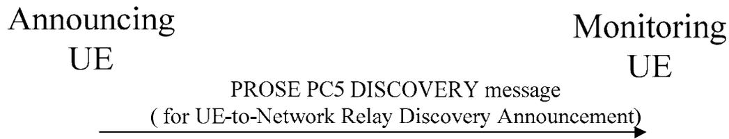
**Figure 8.2.1.2.2.1: Announcing UE procedure for UE-to-network relay discovery**
