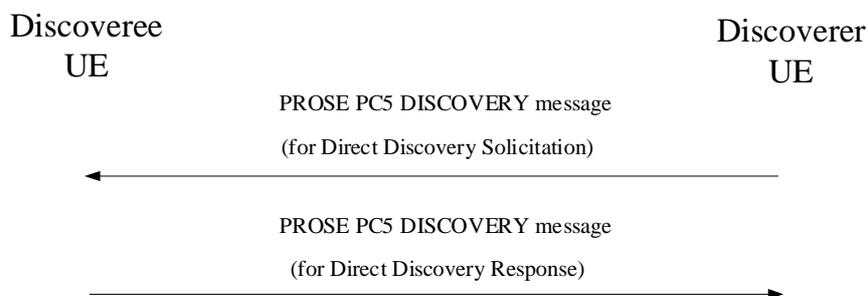
**Figure 6.2.14.2.2.4.1: Discoverer UE procedure for 5G ProSe direct discovery**
