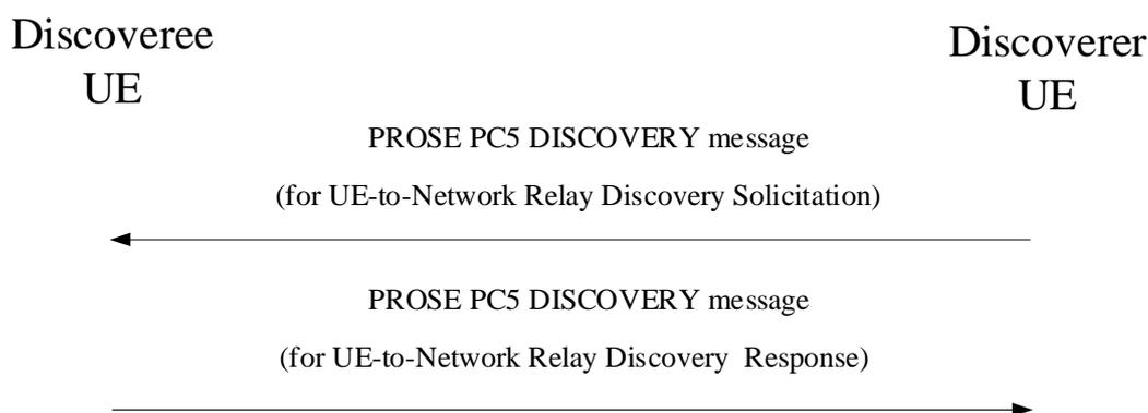
**Figure 8.2.1.3.2.2.1: Discoveree UE procedure for UE-to-network Relay discovery**
