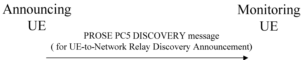
Figure 8.2.1.2.3.2.1: Monitoring UE procedure for UE-to-network relay discovery
