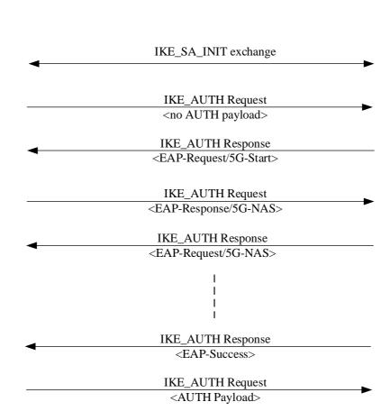
Figure 7.3.2.2-1: IKE SA and first child SA establishment procedure for UE registration over non-3GPP access
