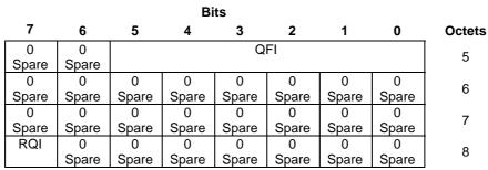
Figure 9.3.3-3: Key field of GRE header
