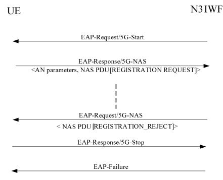
Figure 7.3.3.3-1: EAP-5G session when the UE's registration over non-3GPP access is rejected
