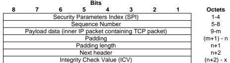
Figure 8.2.2-1: ESP packet format for TCP packet establishing or releasing TCP connection
