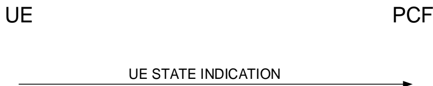
Figure D.2.2.2.1: UE-initiated UE state indication procedure
