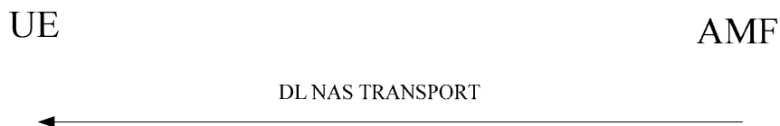
Figure 5.4.5.3.2.1: Network-initiated NAS transport procedure
