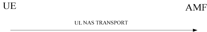
Figure 5.4.5.2.2.1: UE-initiated NAS transport procedure
