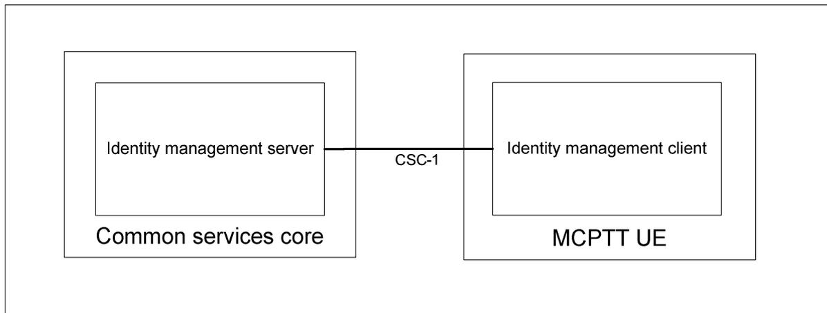
**Figure 4.1-1: Functional model for MCPTT identity management**
