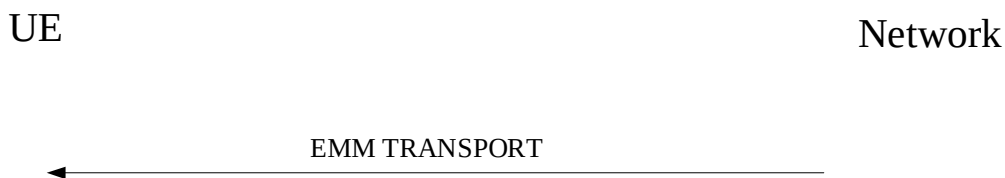
Figure 5.6.5.3.1: Network initiated EMM data transport procedure
