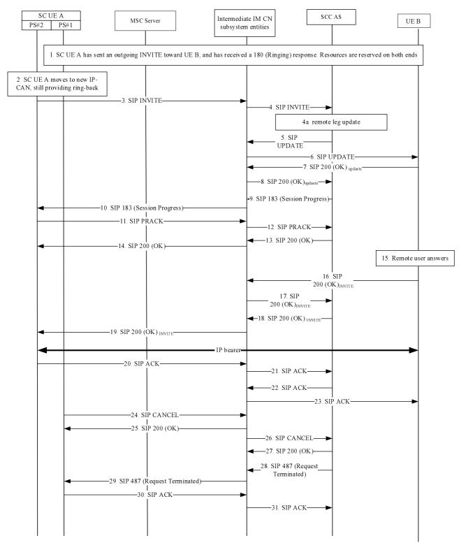
NOTE 3: For clarity, the SIP 100 (Trying) responses are not shown in the signalling flow.
