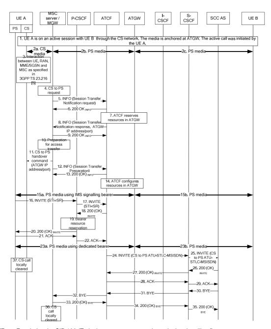
NOTE: For clarity, the SIP 100 (Trying) responses are not shown in the signalling flow. Figure A.20.2-1 Signalling flows for CS to PS Access Transfer: CS to PS SRVCC occurs during a call.
