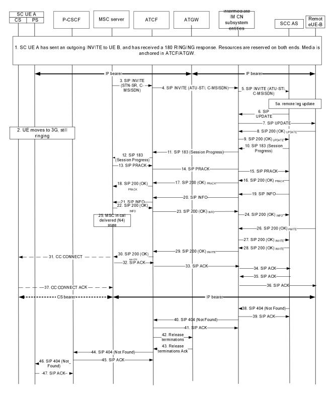
NOTE: For clarity, the SIP 100 (Trying) responses are not shown in the signalling flow. Figure A.18.4-1: PS-CS SRVCC, originating call in alerting phase
