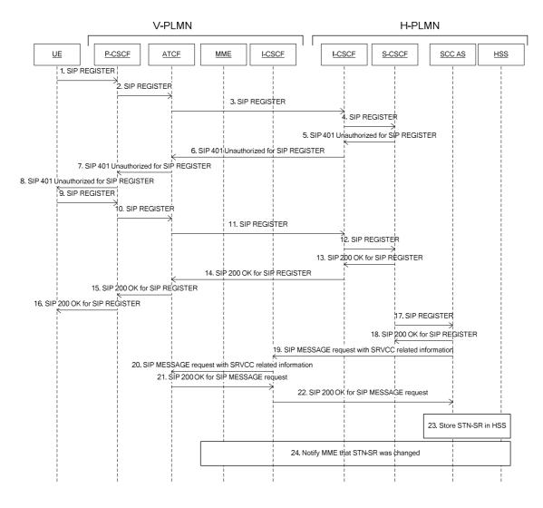
Figure A.3.3-1 registration with SRVCC enhancements
