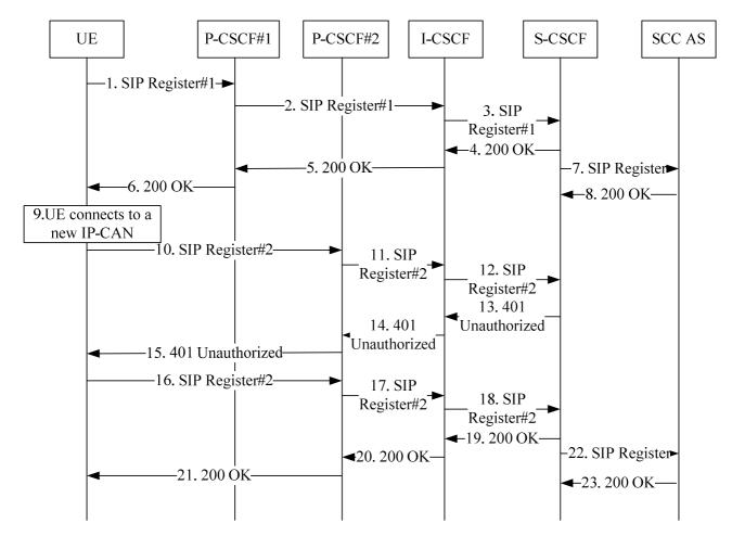
Figure A.3.2-1 Signalling flows for multiple registrations
