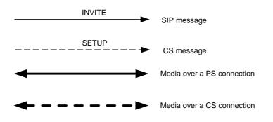
Figure A.2-1: Signalling flow notation
