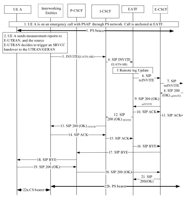
Figure A.17.3-1 Signalling flow for emergency session transfer using SRVCC procedure
