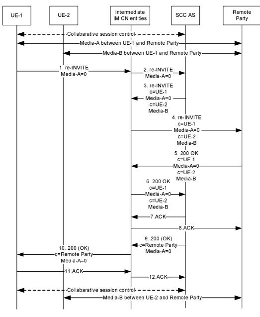
Figure A.15.3.1: Controller UE releases media flow on controller UE
