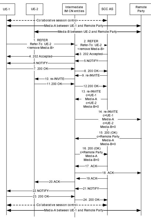
Figure A.15.3.2.1:Controller UE remove media at the controllee UE
