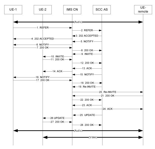
Figure A.12.3: Controller UE establishes a collaborative session by adding a new media on controllee UE
