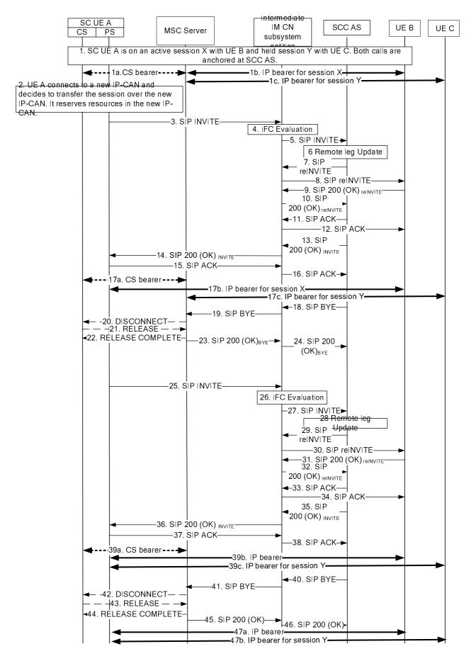
Figure A.16.2-1: Signalling flow for PS-CS Access Transfer: CS to PS
