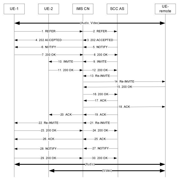
Figure A.13.2: Controller UE transfers a media on controllee UE
