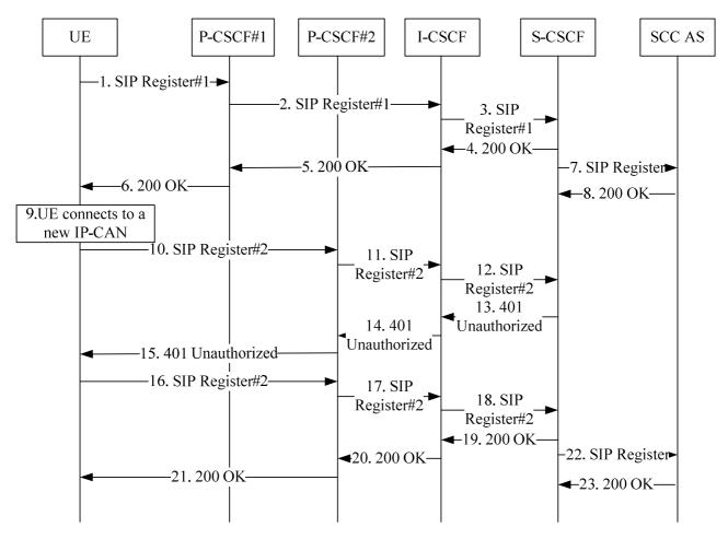
Figure A.3.2-1 Signalling flows for multiple registrations
