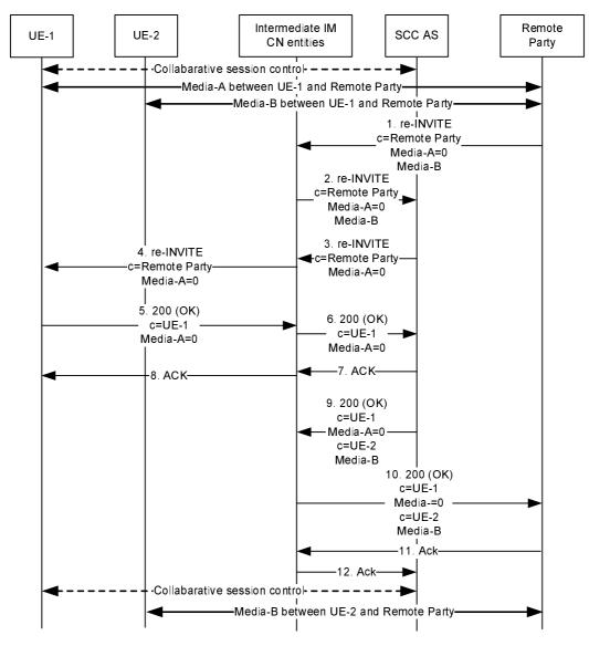
Figure A.15.7: Remote UE releases media on the Controller UE
