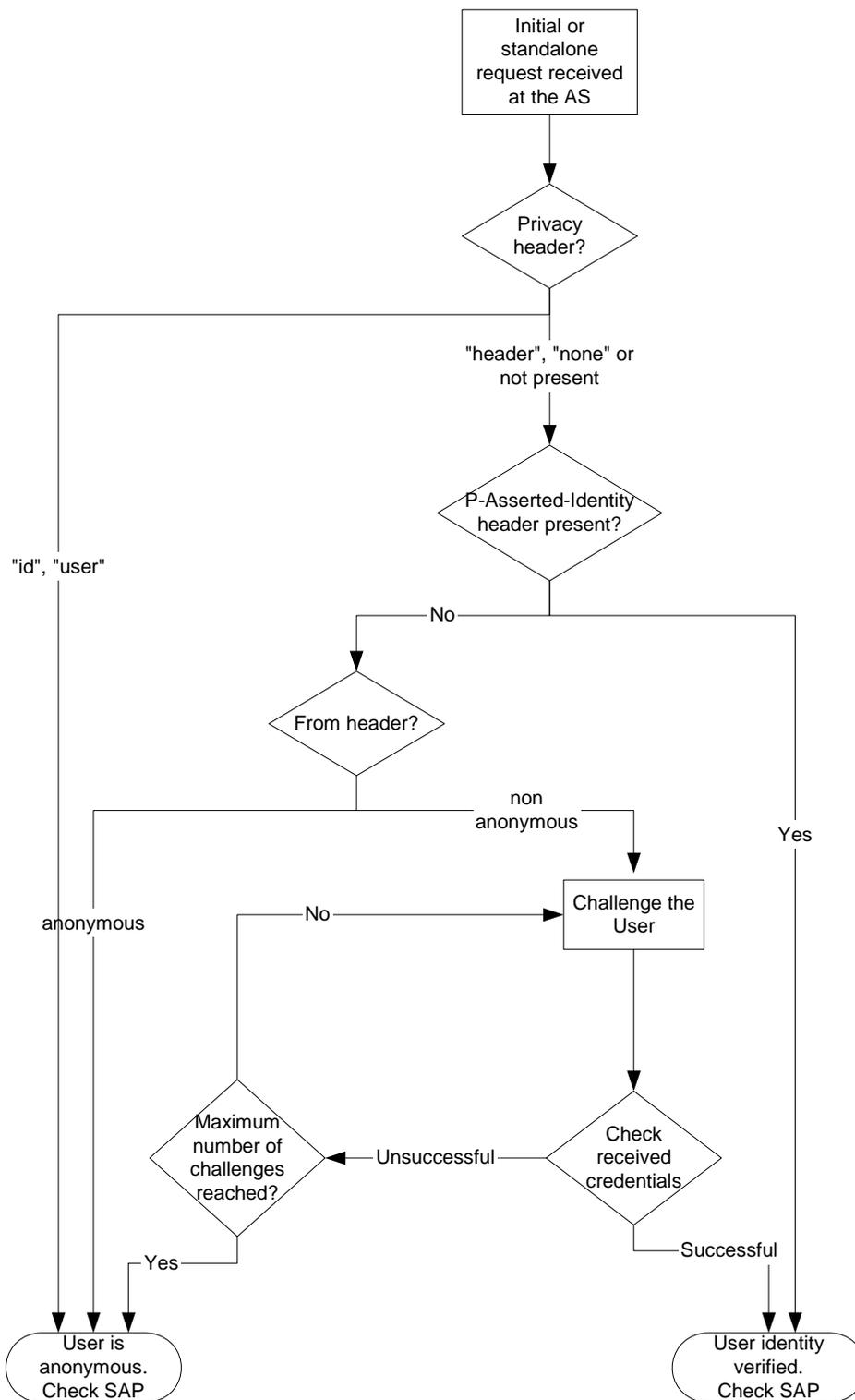
Figure 5-1: User identity verification flow at the AS
