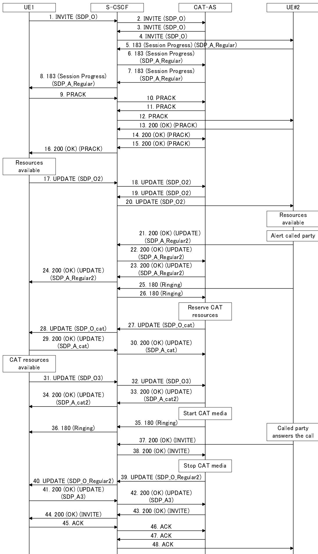
**Figure A.5.8-1: CAT with different media types during one session, UE#1 and UE#2 does not have required resources available**
