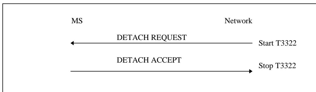
Figure 4.7.4/2 3GPP TS 24.008: Network initiated GPRS detach procedure
