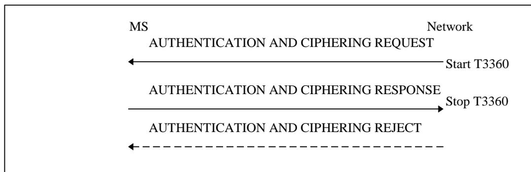
**Figure 4.7.7/1 3GPP TS 24.008: Authentication and ciphering procedure**
