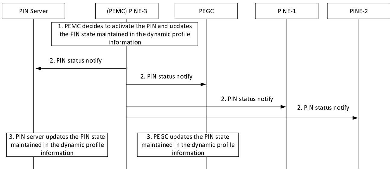
**Figure 8.5.13.2.1-1: Activation of PIN by PEMC**
