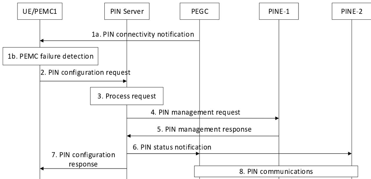
**Figure 8.5.10.2.2-1: PIN Modification after local PEMC failure**
