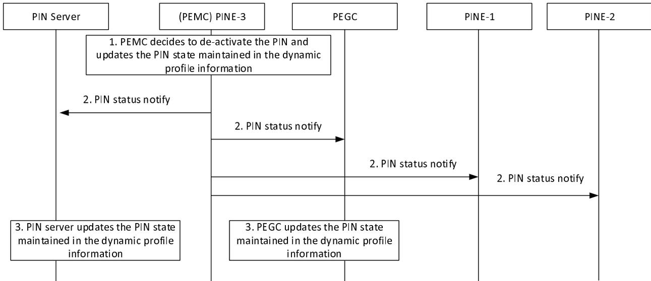
**Figure 8.5.13.2.2-1: Deactivation of PIN by PEMC**
