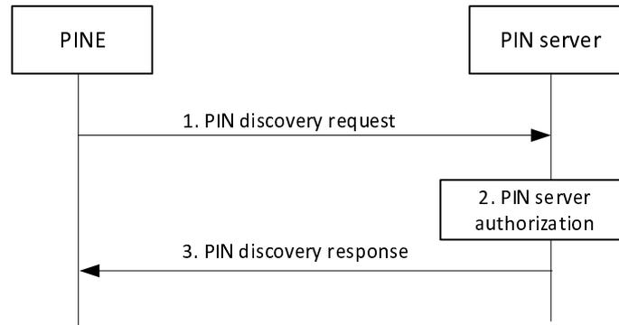
**Figure 8.5.7.2.2-1: PIN discovery based on PIN server**
