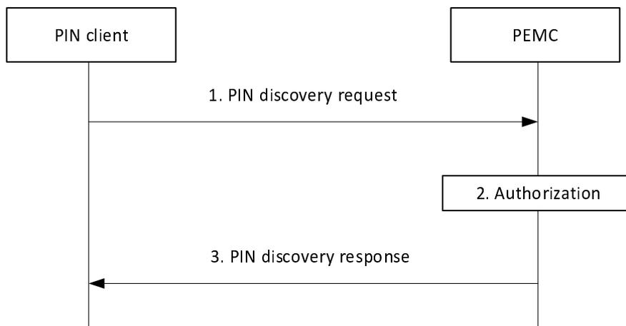
**Figure 8.5.7.2.1-1: Procedures of PIN discovery based on PEMC**
