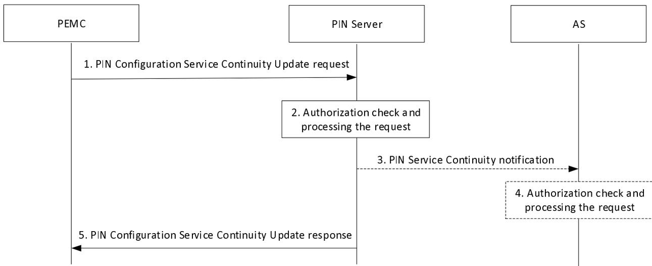
**Figure 8.9.2.1.4-1: PIN Configuration Update procedure**
