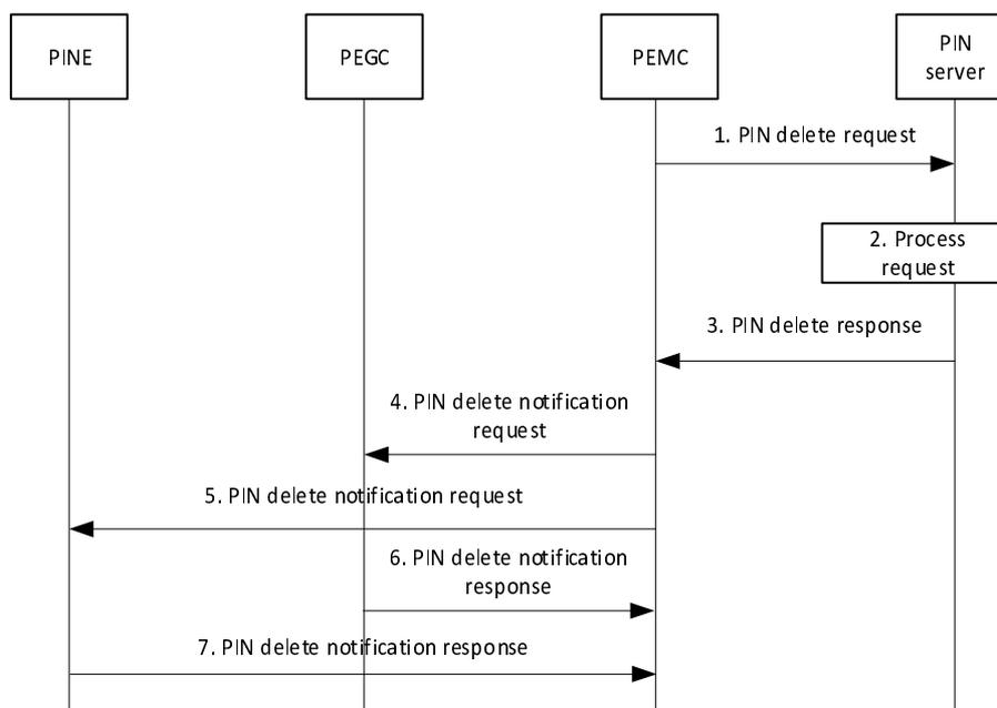
**Figure 8.5.3.2.1-1: PIN delete procedure involving PIN server**
