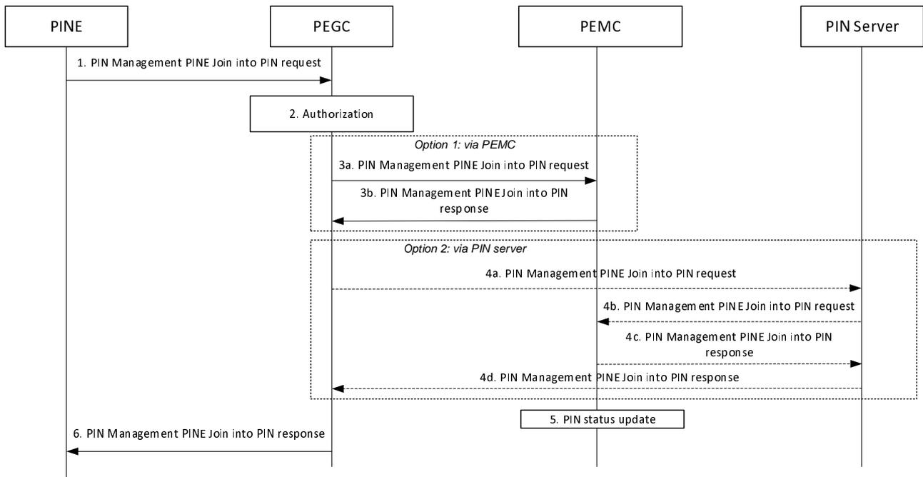
**Figure 8.5.8.2.4-1: PINE join into PIN via PEGC**
