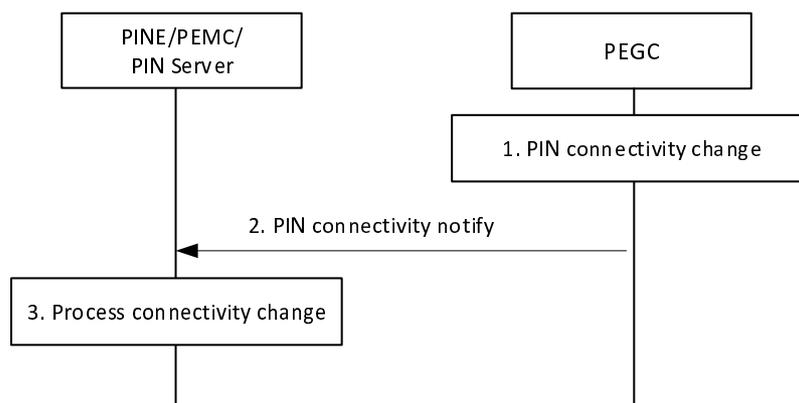
**Figure 8.5.14.2.2-1: PIN connectivity notify procedure**
