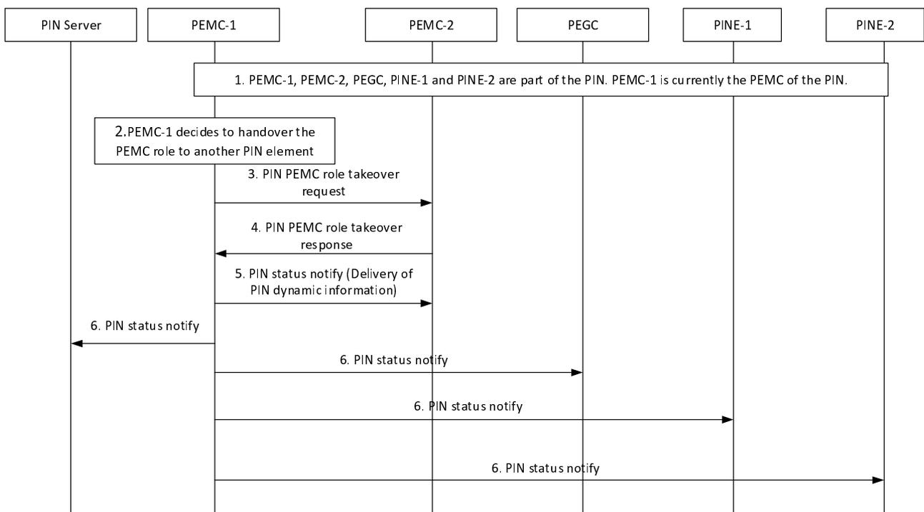
Figure 8.5.2.10.2-4-1: PEMC replacement triggered internally within the PIN
