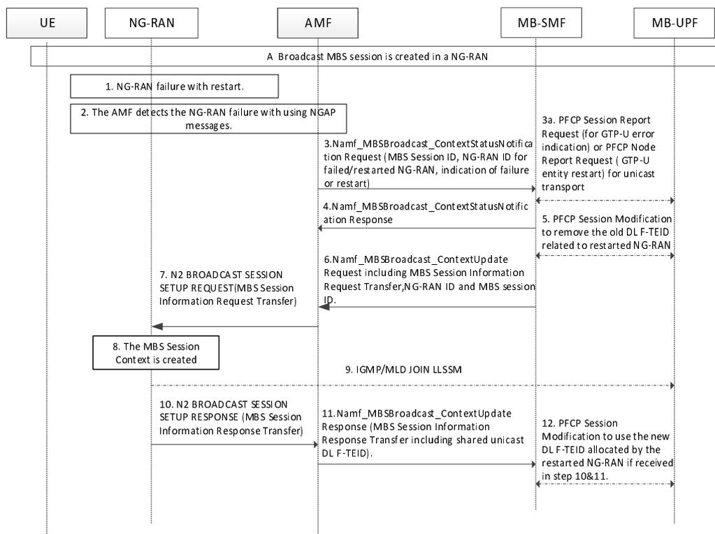
**Figure 8.3.2.3-1: Broadcast MBS session restoration by MB-SMF upon NG-RAN failure with restart**
