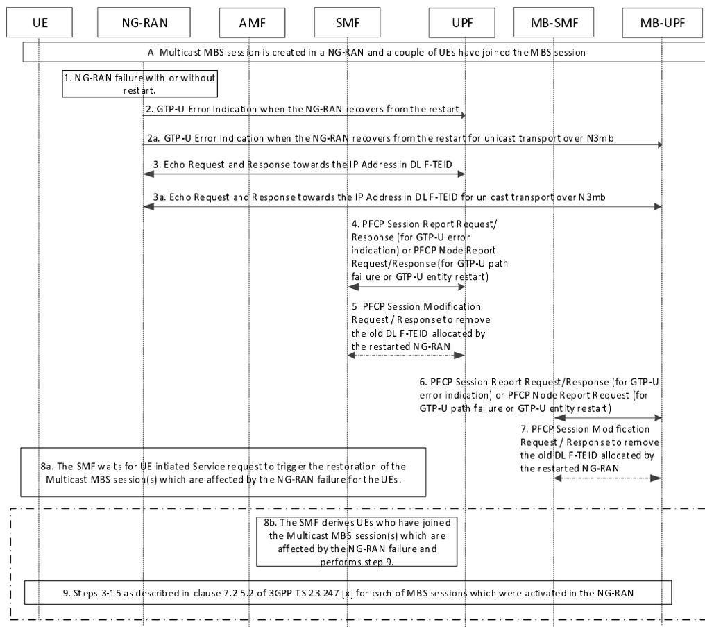
Figure 8.3.4-1: Multicast MBS session restoration upon NG-RAN failure with or without restart
