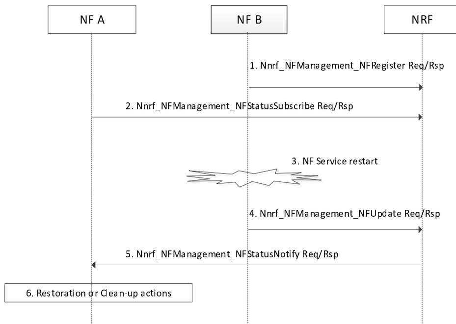
**Figure 6.2.3-2: NF Service Restart Detection and Notification**
