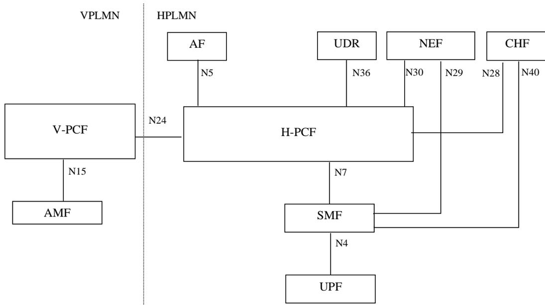
**Figure 5.2.2-2a: Overall roaming reference architecture of policy and charging control framework for the 5G System - home routed scenario (reference point representation)**
