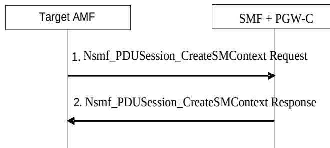
Figure 4.11.1.4.2-1: Procedures for EPS bearer IDs transfer
