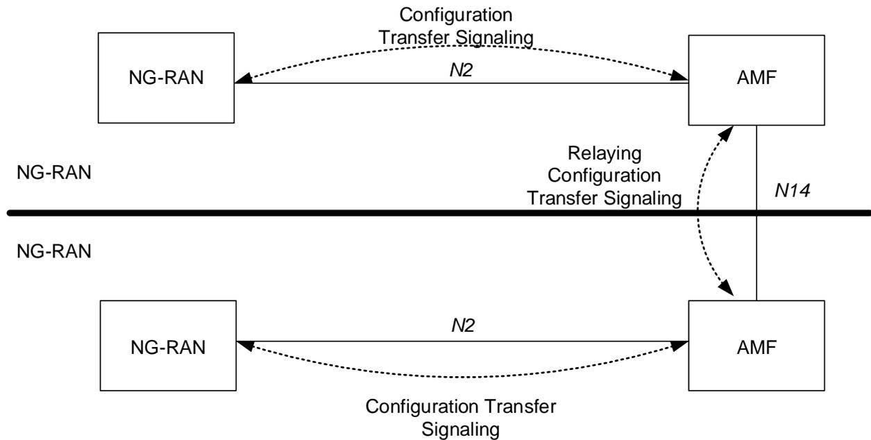
**Figure 5.26-1: inter NG-RAN Configuration Transfer basic network architecture**
