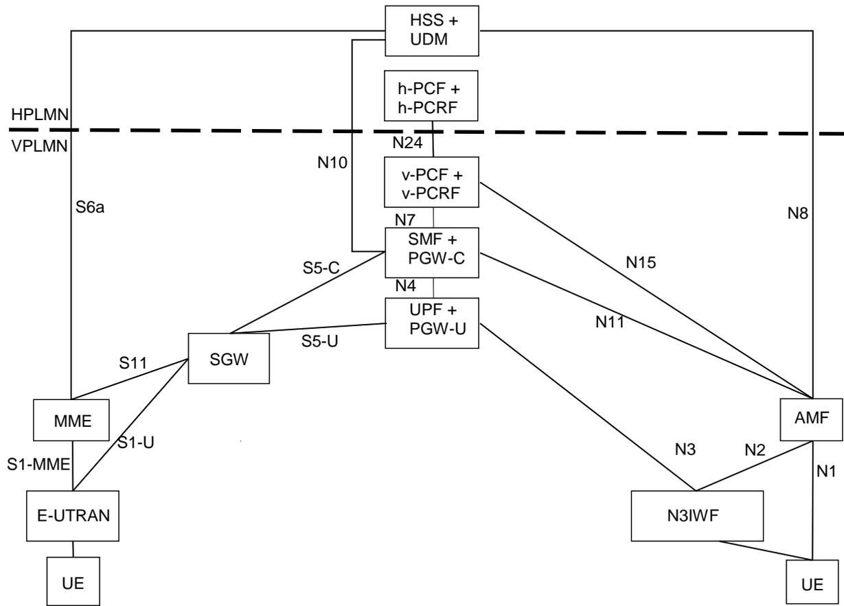
**Figure 4.3.3-1: Local breakout roaming architecture for interworking between 5GC via non-3GPP access and EPC/E-UTRAN**
