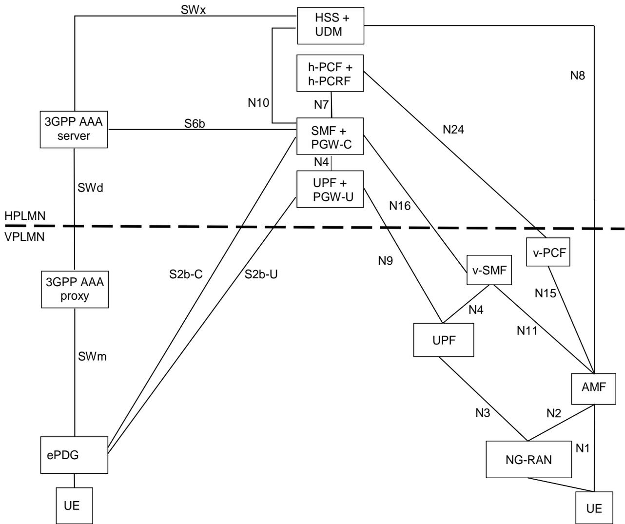
**Figure 4.3.4.2-2: Home-routed roaming architecture for interworking between ePDG/EPC and 5GS**
