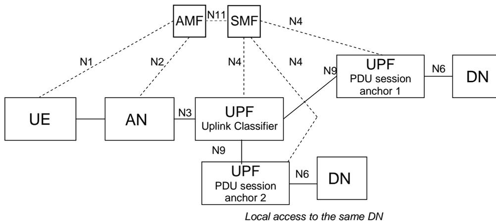
**Figure 5.6.4.2-1 User plane Architecture for the Uplink Classifier**
