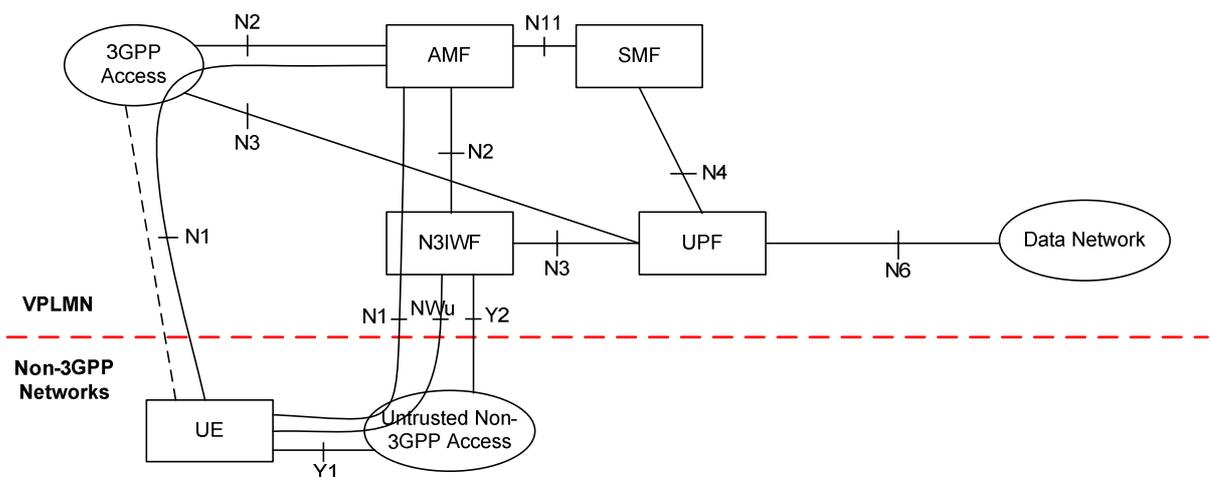
Figure 4.2.8.2.2-1: LBO Roaming architecture for 5G Core Network with non-3GPP access - N3IWF in the VPLMN
