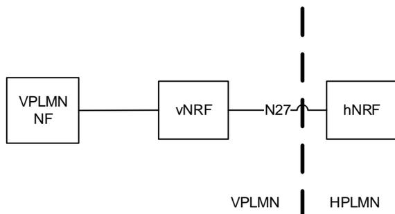
**Figure 4.2.4-7: NRF Roaming architecture in reference point representation**
