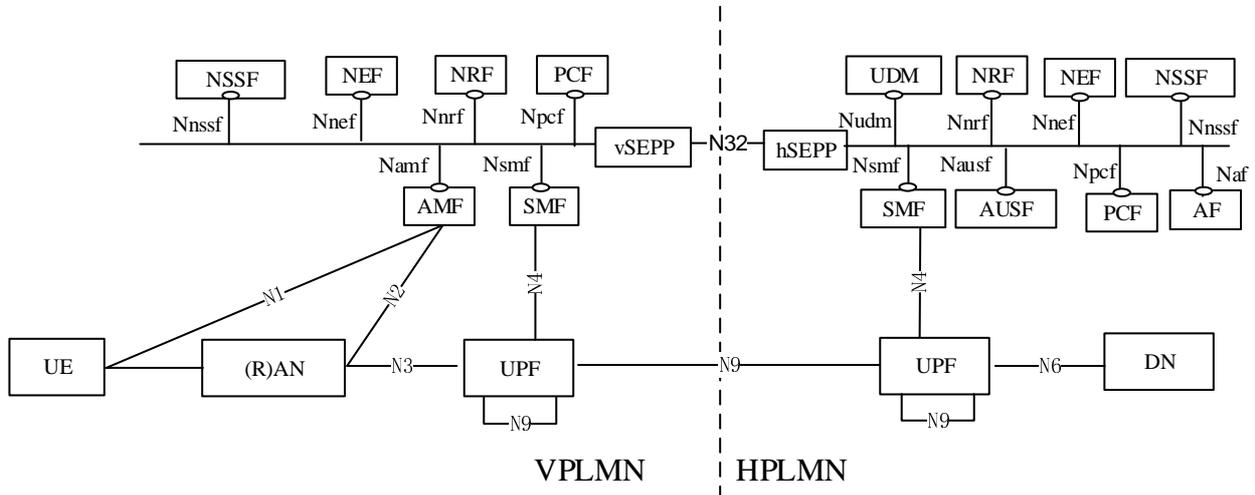
Figure 4.2.4-3 Roaming 5G System architecture - home routed scenario in service-based interface representation
