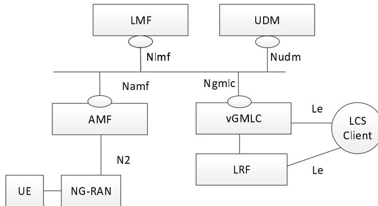
**Figure 4.4.4.1-1: Non-roaming reference architecture for Location Services**
