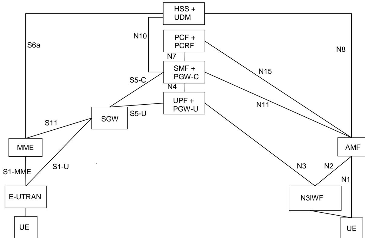
**Figure 4.3.3-1: Non-roaming architecture for interworking between 5GC via non-3GPP access and EPC/E-UTRAN**
