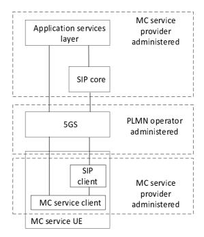
Figure 6.3.1.4-1: MC service provider provision of SIP core, separate domain from 5GS
