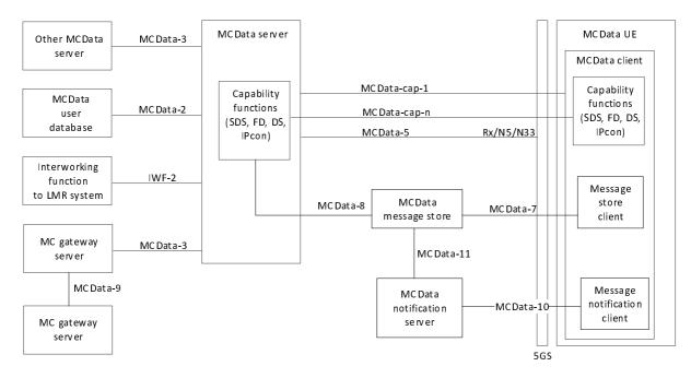
Figure 5.6.1-1: Generic MCData functional model for application plane
