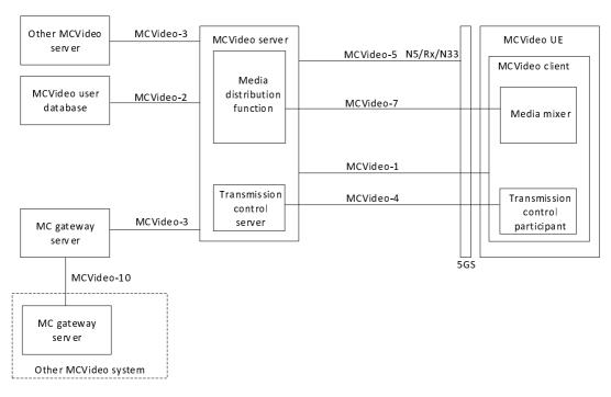
Figure 5.5.1-1: MCVideo functional model for application plane
