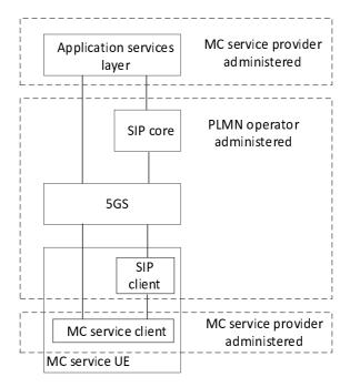
Figure 6.3.1.3-1: MC service provider administers MC service separately from SIP core and 5GS
