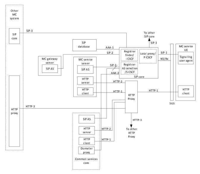
Figure 5.3.1-2: Common functional model for signalling control plane
