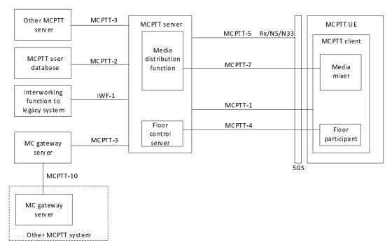
Figure 5.4.1-1: MCPTT functional model for application plane
