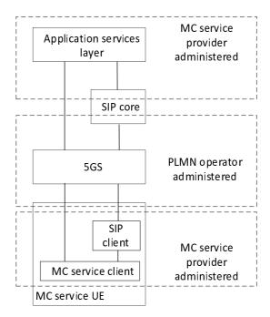
Figure 6.3.1.5-1: MC service provider partial provision of SIP core, separate domain from 5GS
