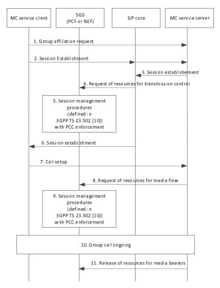
Figure 7.2.5.2-1: Request of resources for transmission control and media plane
