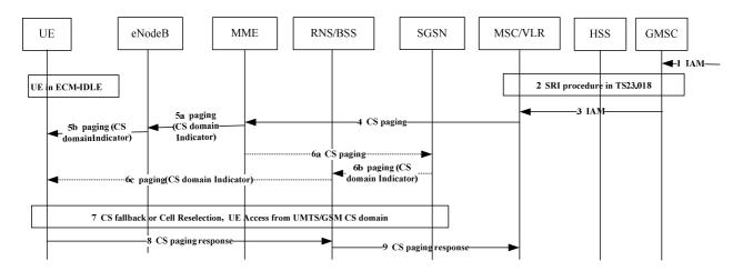
Figure 7.7.2-1: Mobile Terminating Call when ISR is active and SGs is active between MSC/VLR and MMF
