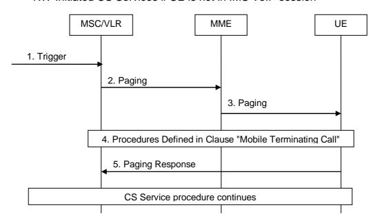
Figure 8.4.2.1-1: NW-Initiated CS Service procedure
