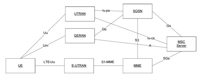
Figure 4.2-1: EPS architecture for CS fallback and SMS over SGs
