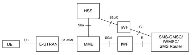
Figure C.2-2: SMS in MME architecture using IWF
