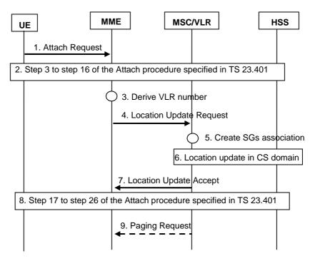
Figure 5.2-1: Attach Procedure
