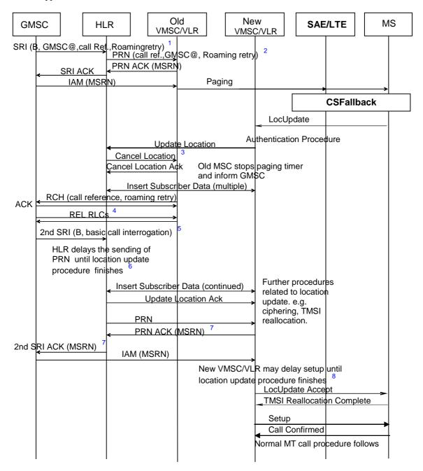
Figure 7.5-1: Roaming Retry for CS fallback
