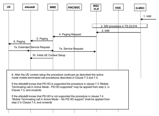
Figure 7.2-1: Mobile Terminating Call in idle mode
