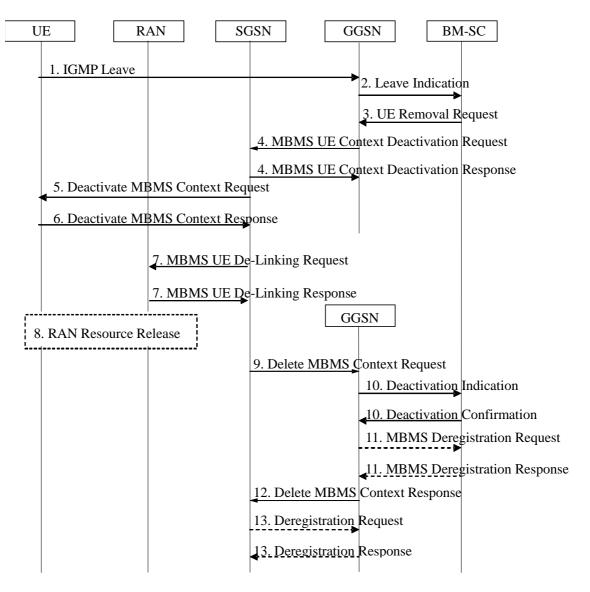
Figure 13: MBMS Multicast Service Deactivation
