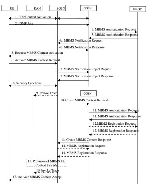
Figure 7: The activation of an MBMS multicast service
