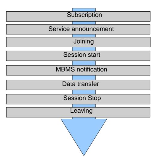
Figure 2: Phases of MBMS Multicast service provision
