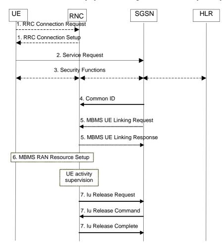
Figure 17: MBMS Service Request procedure
