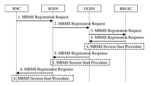
Figure 9: MBMS Registration procedure
