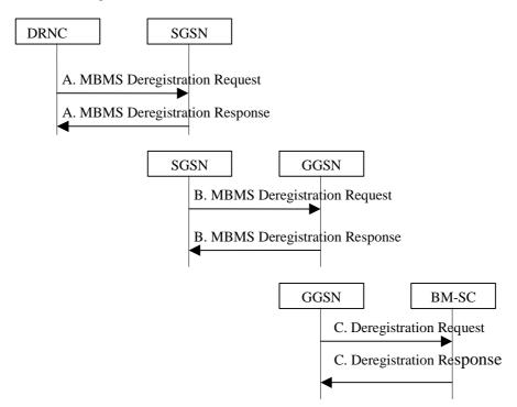
Figure 11: MBMS De-Registration Procedure
