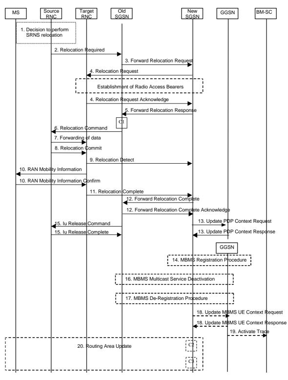
Figure 15: SRNS Relocation Procedure
