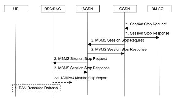
Figure 10: MBMS Session Stop procedure for GERAN and UTRAN for GPRS
