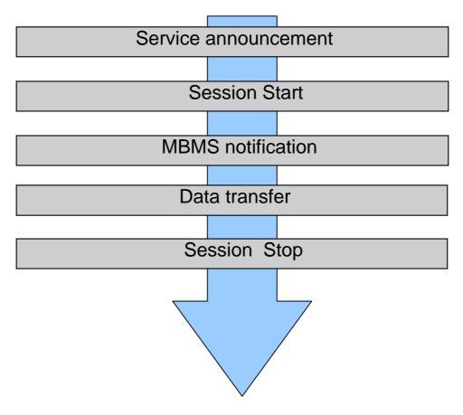
Figure 4: Phases of MBMS broadcast service provision
