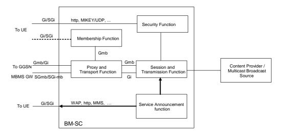
Figure 5a: BM-SC functional structure
