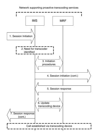
Figure P.1.3.2-1: Proactive transcoding triggering logic
