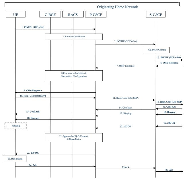
Figure N.1.1: Fixed xDSL originating - home (example flow)
