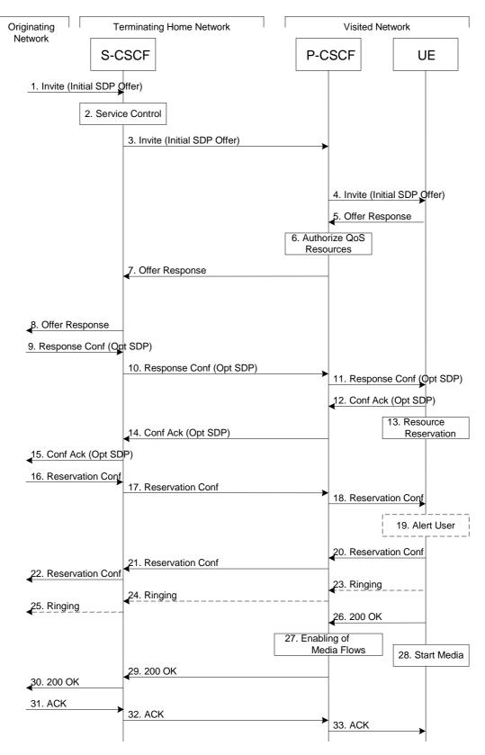
Figure 5.17: Mobile termination procedure - roaming
