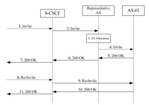
Figure J.2.2: Bypassing Representative AS procedure
