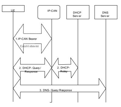
Figure 5.0a: P-CSCF discovery using DHCP and DNS
