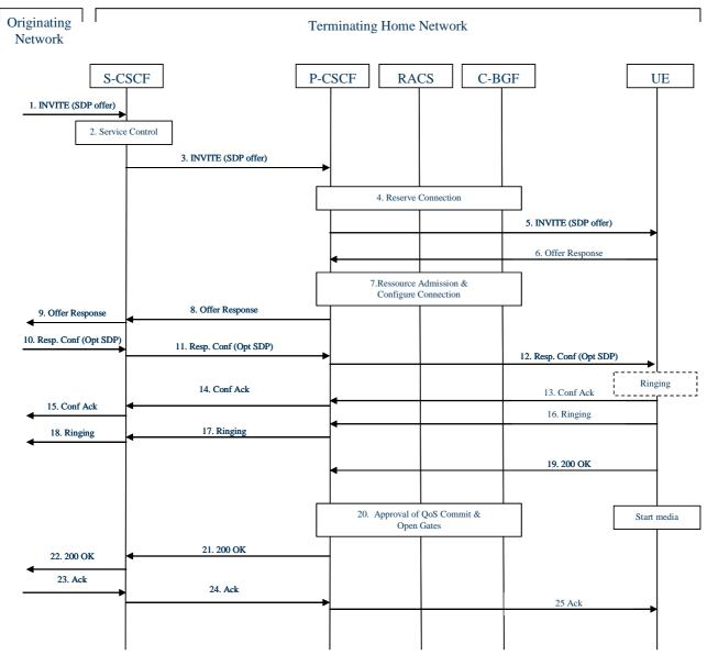
Figure N.2.1: Fixed xDSL terminating - home (example flow)
