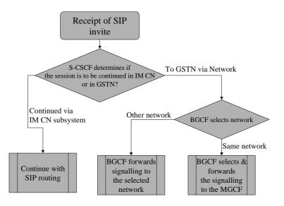
Figure 5.6: Network based PSTN interworking breakout process
