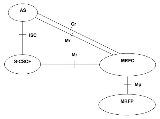
Figure 4.7: Architecture of MRF
