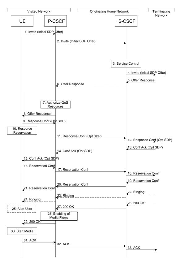
Figure 5.14: Mobile origination procedure - roaming
