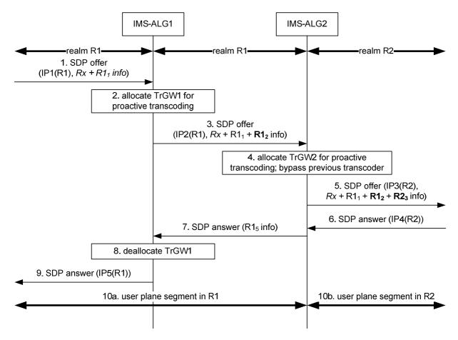
Figure Q.8: IMS-ALG replaces prior proactive transcoder
