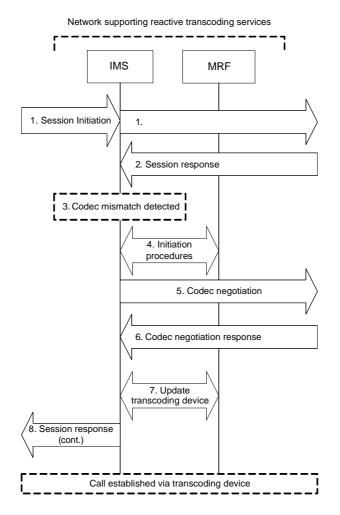
Figure P.1.3.3-1: Reactive transcoding triggering logic
