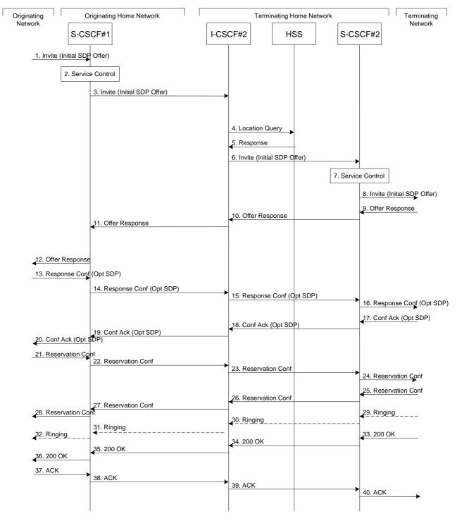
Figure 5.10: Serving to serving procedure - different operators
