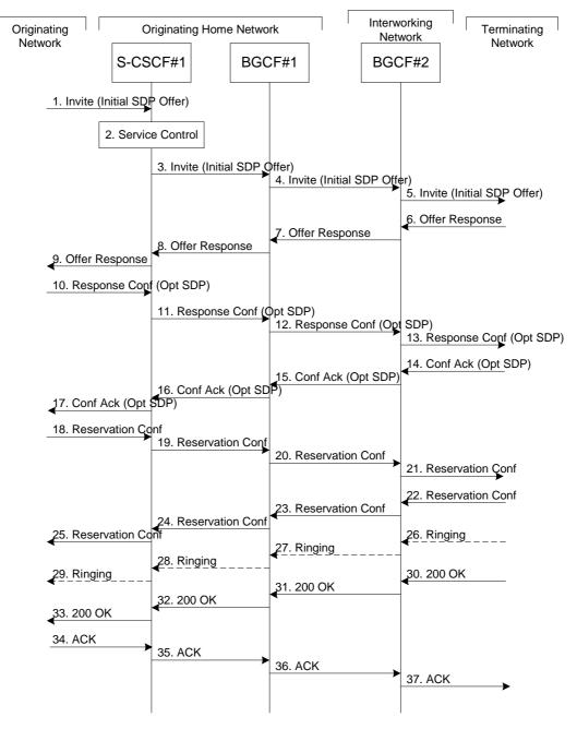
Figure 5.13: Serving to PSTN procedure - different operator
