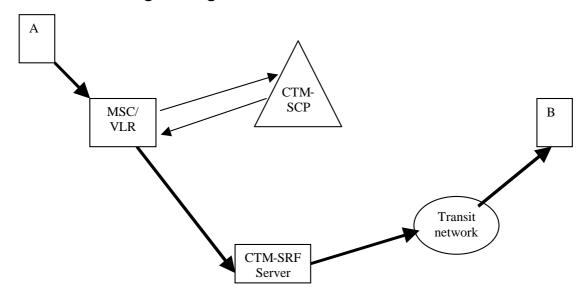
Figure C.4: Mobile originating call routing overview
