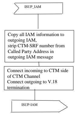
Figure C.10: Routing logic in CTM-SRF, for Mobile Originated calls
