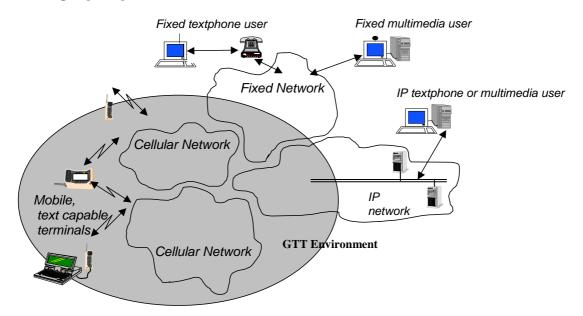
Figure 1: General view of GTT feature provision within the different networks
