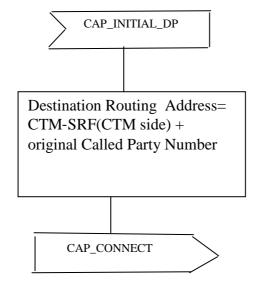
Figure C.8: CTM\_SCP logic for Mobile Originated case at detection point=Collection of dialled digits
