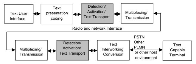
Figure 3: GTT general text transmission functions showing interworking
