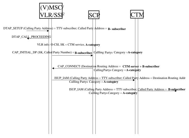
Figure C.6: Mobile Originating Text Call
