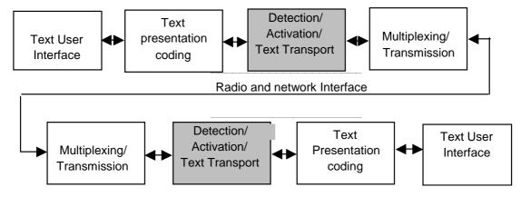
Figure 2: Call flow for two mobile terminals with the same GTT transport method, using text conversation
