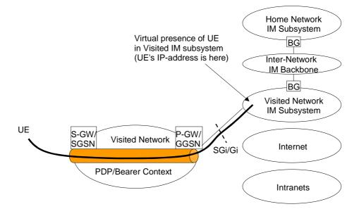
Figure 5-5: UE Accessing IM Subsystem Services with P-GW/GGSN in the Visited network via Visited Network IM subsystem
