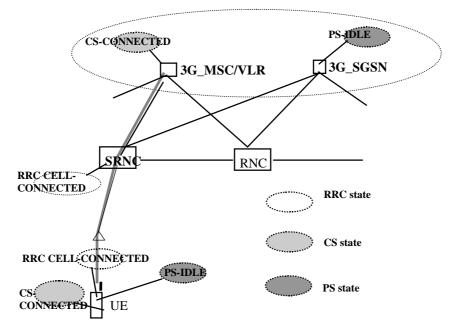
Figure 6.5: UE in CS-CONNECTED state and PS-IDLE state
