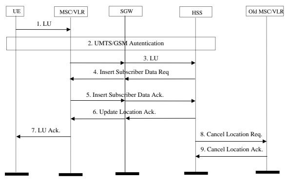
Figure 8.3: Message sequence for roaming into a CS domain
