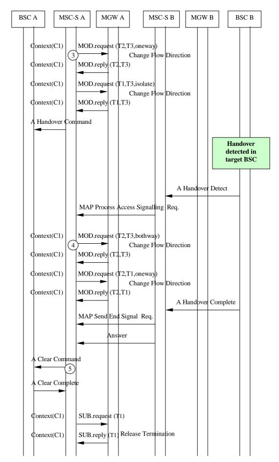
Figure 8.22/2: Basic Inter-MSC GSM to GSM Handover (message sequence chart)
