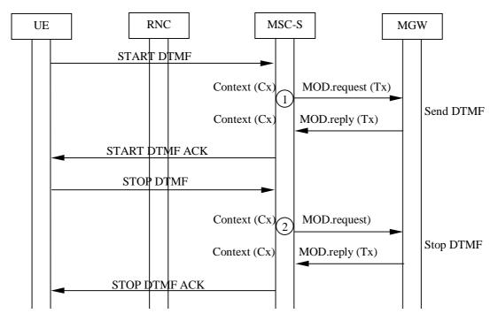
Figure 14.3: Inband DTMF generation (message sequence chart)
