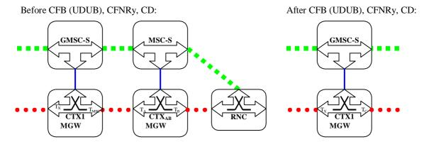
Figure 14.9: Optimal routeing; late call forwarding (CFB (UDUB), CFNRy, CD) (Network model)
