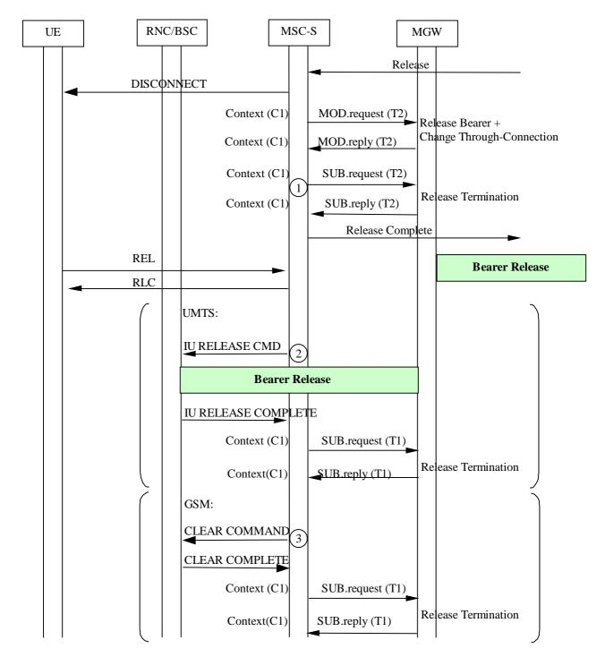
Figure 7.2: Network Initiated Call Clearing (message sequence chart)
