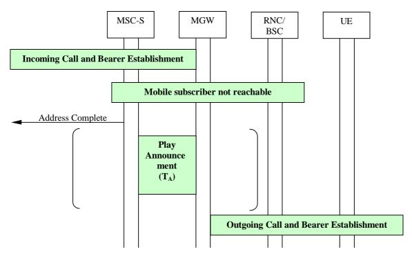
Figure 13.12: CFNRc (Rerouting by VLR) (message sequence chart)
