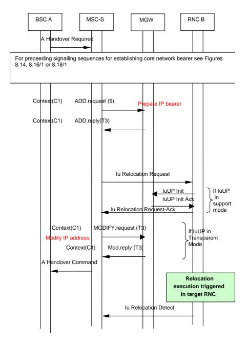
Figure 8.3.5/1 GSM to UMTS Handover with lu on IP
