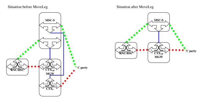
Figure 14. 1.3/3 Move Leg procedure (Network model)
