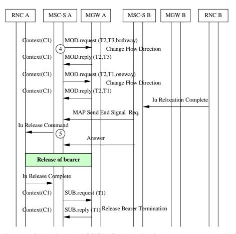
Figure 8.4/2: Basic Inter-MSC SRNS Relocation (message sequence chart)
