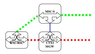
Figure 7.7: MGW Initiated Call Clearing (Network model)
