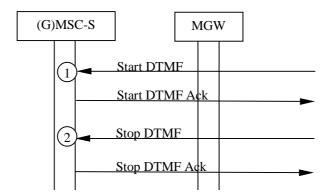
Figure 14.6: Out-of-Band DTMF detection (message sequence chart)
