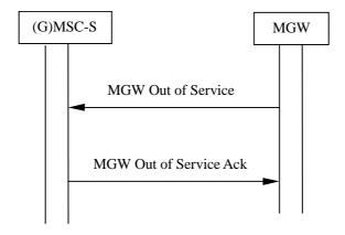
Figure 10.2: MGW indicates the Failure/Maintenance locking
