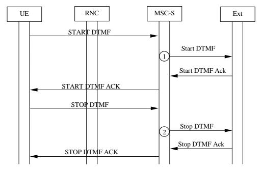
Figure 14.4: Out-of-Band DTMF generation (message sequence chart)
