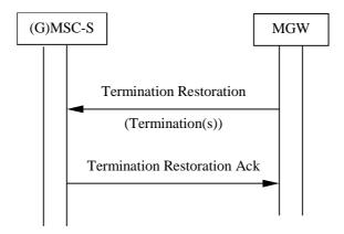
Figure 10.10: Restoration to service of a Physical Termination
