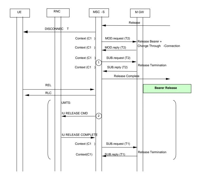
Figure 7.10 Network Initiated Call Clearing (message sequence chart)
