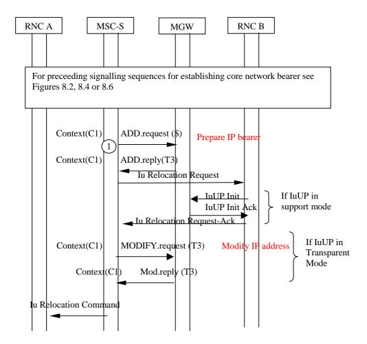
Figure 8.1.5/1 SRNS Relocation with lu on IP
