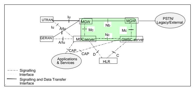
Figure 1: CS core network logical architecture
