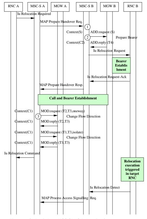
Figure 8.4/1: Basic Inter-MSC SRNS Relocation (message sequence chart)
