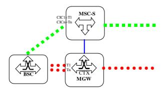
Figure 9.1 TDM circuits used for A-interface (network model)
