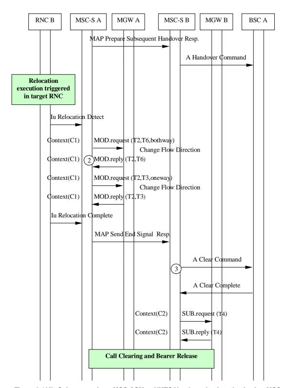
Figure 8.18/2: Subsequent Inter-MSC GSM to UMTS Handover back to the Anchor MSC (message sequence chart)
