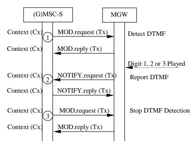
Figure 14.5: Inband DTMF detection (message sequence chart)
