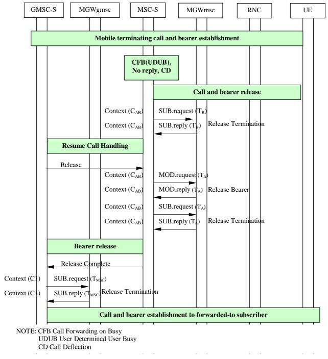
Figure 14.11: Optimal call routeing; late call forwarding (CFB (UDUB), CFNRy, CD), backward bearer release (message sequence chart)
