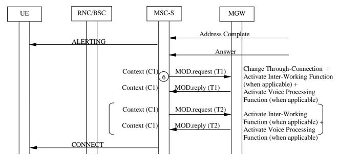
Figure 6.2/2: Basic Mobile Originating Call, Forward Bearer Establishment (message sequence chart continue)
