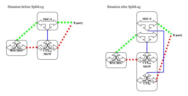
Figure 14. 1.3/5 Split Leg procedure (Network model)
