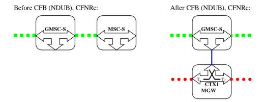
Figure 14.7: Optimal routeing; late call forwarding (CFB (NDUB), CFNRc) (Network model)
