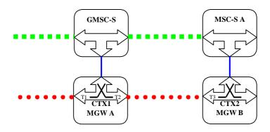
Figure 18.1A: MSC before MGW Tandeming during call setup to provide bearer access to specialised MGW resources (Network model)
