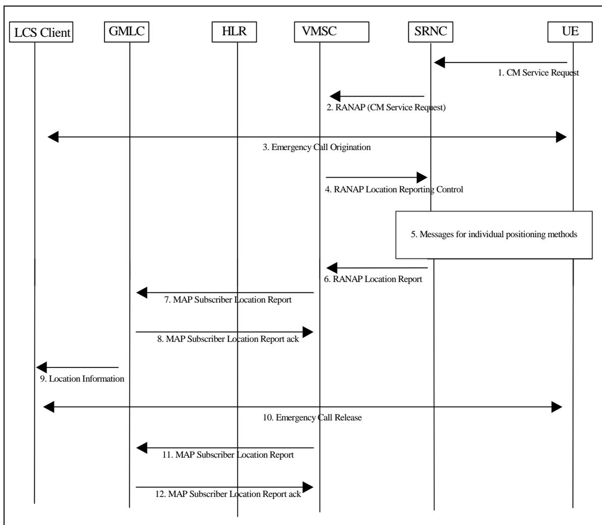
Figure 8.5: Positioning for a NI-LR Emergency Service Call
