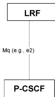
**Figure C.1: Additional P-CSCF interface for fixed broadband access**
