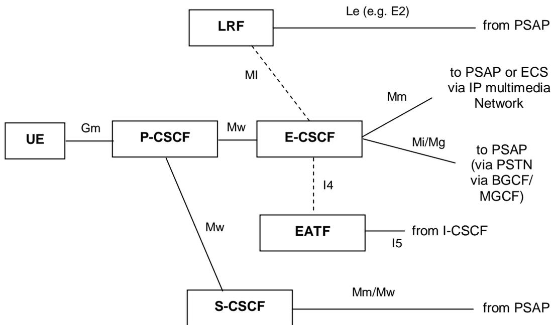
**Figure 5.1: E-CSCF in reference architecture**
