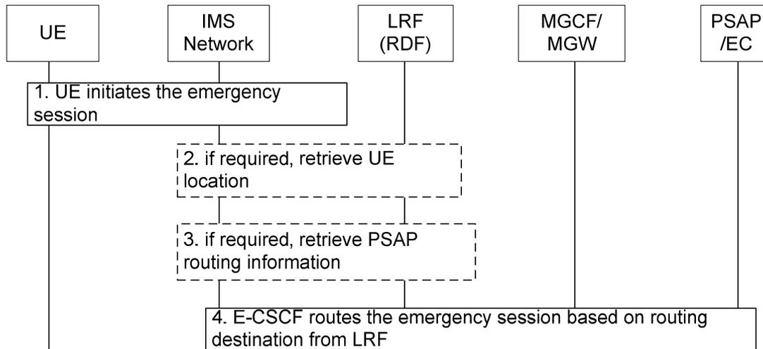
**Figure 7.2: Emergency Session Establishment procedure with using LRF/RDF**
