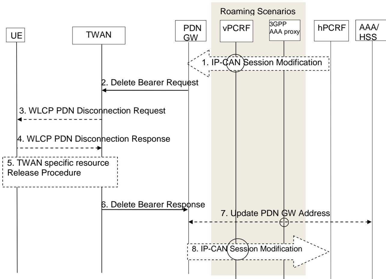
**Figure 6.5.2.2-2: Network-initiated Removal of Trusted WLAN access from the PDN connection**
