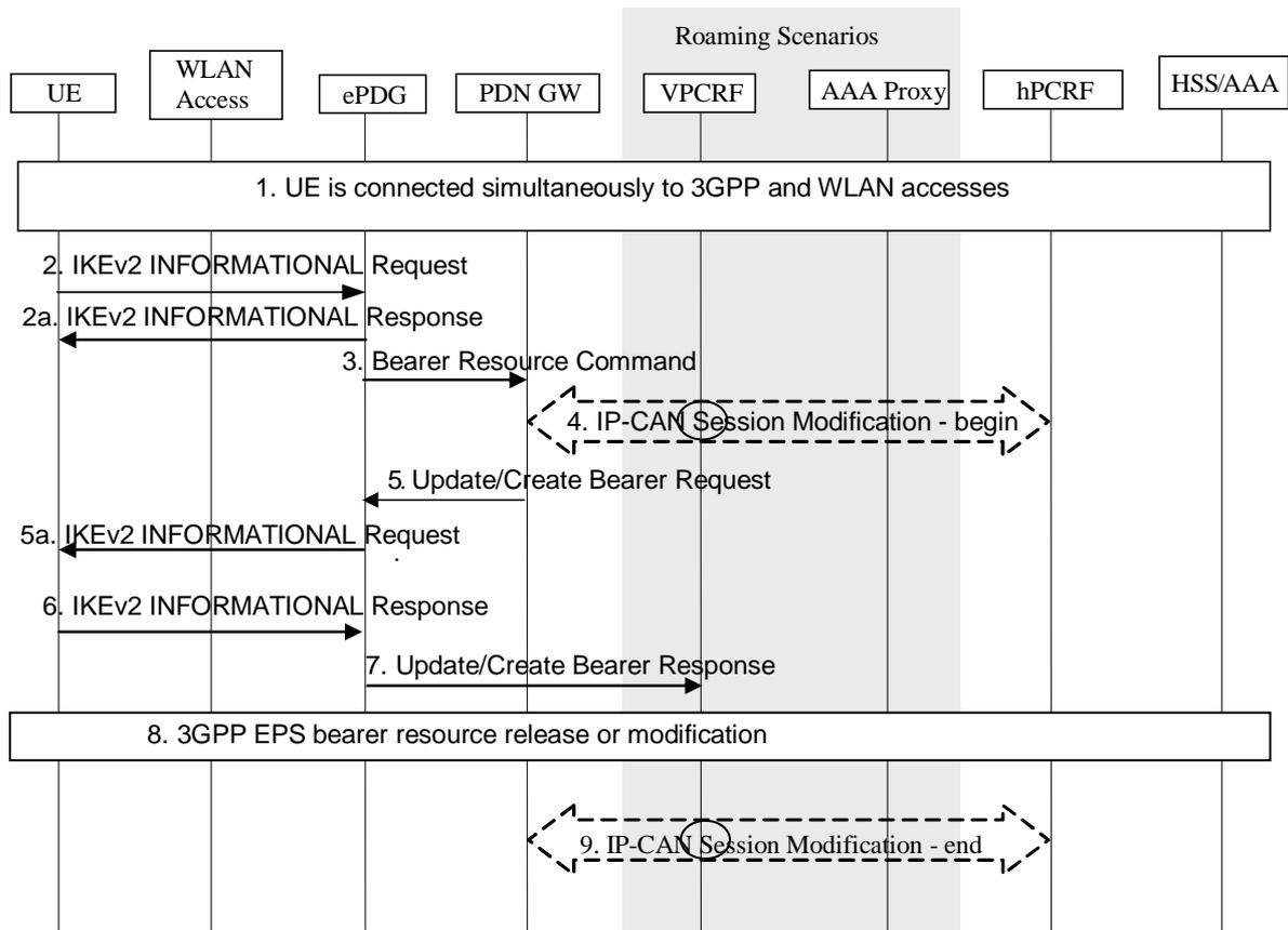
**Figure 6.3.3.3-1: IP flow mobility within a PDN connection initiated over WLAN access**
