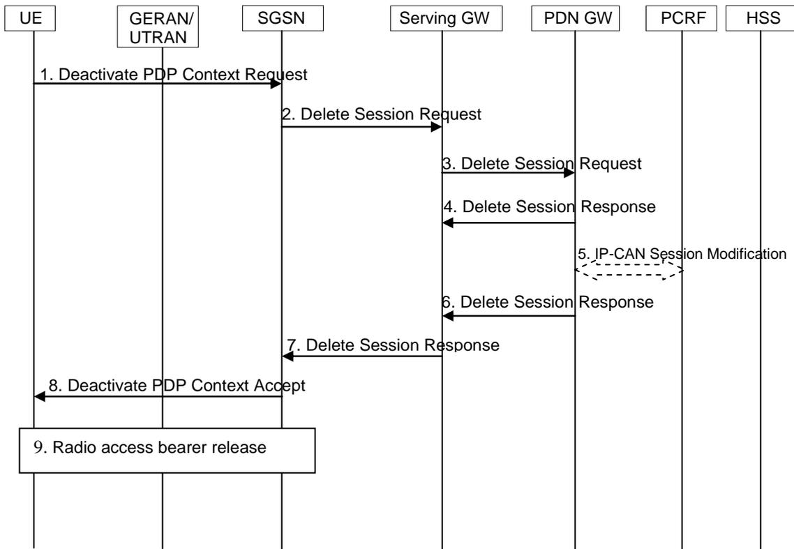
**Figure 6.5.1.1-3: UE-Initiated Removal of 3GPP access via GERAN/UTRAN**
