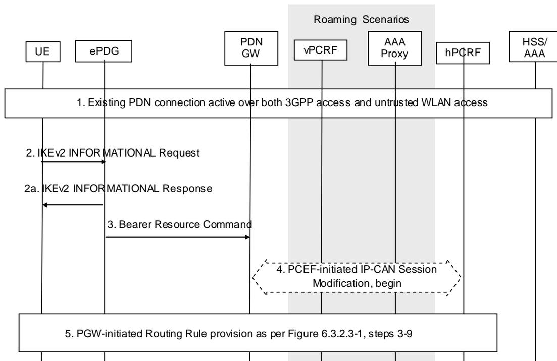
**Figure 6.4.3-1: UE Requested IP Flow Mapping via untrusted WLAN access using GTP**
