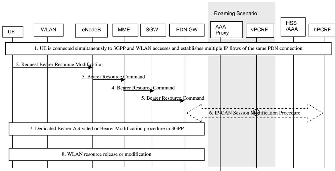
**Figure 6.4.1-1: UE requested IP flow mapping via E-UTRAN**
