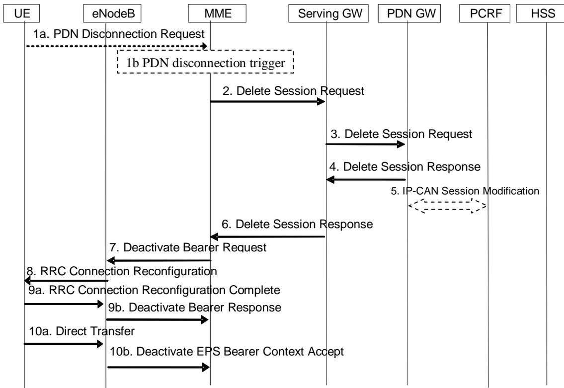
**Figure 6.5.1.1-1: UE-Initiated Removal of 3GPP access via E-UTRAN**
