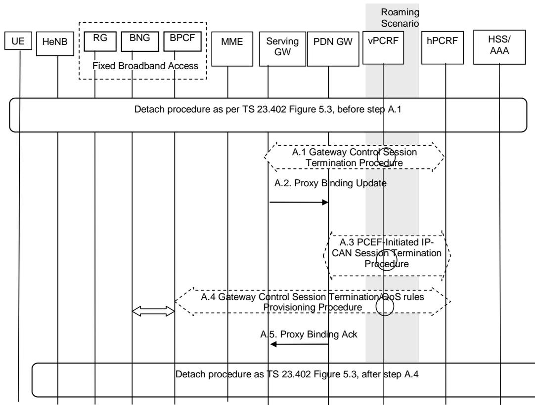
**Figure 9.2.2-1: E-UTRAN Detach Procedure for PMIP-based S5/S8**
