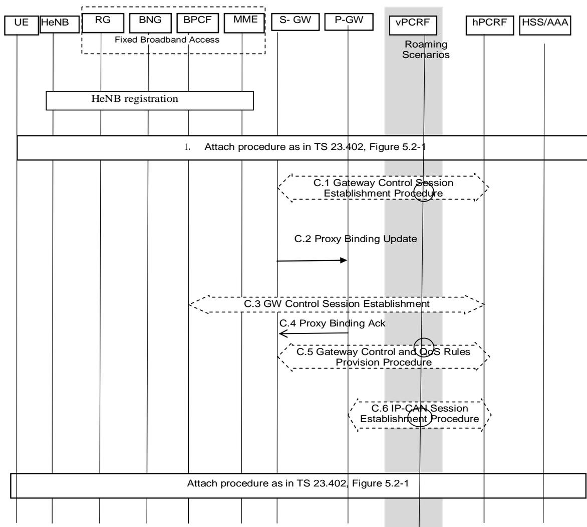
Figure 9.2.1-1 : Initial E-UTRAN attach with PMIP-based S5/S8
