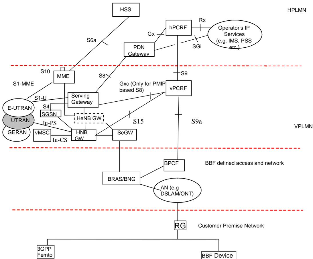
**Figure 4.3.3-1: Roaming Architecture - Home Routed Traffic**
