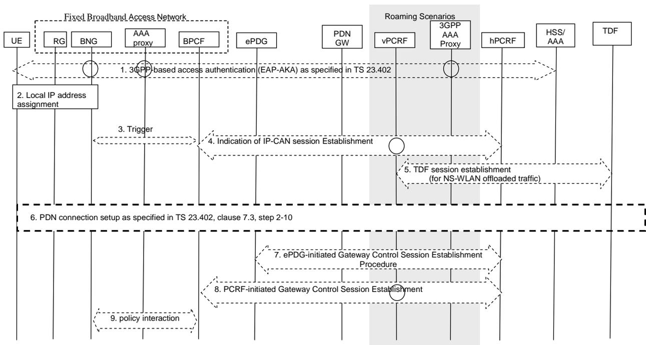
**Figure 8.3.1-1: Initial attachment when S2c is used for roaming, non-roaming and LBO**
