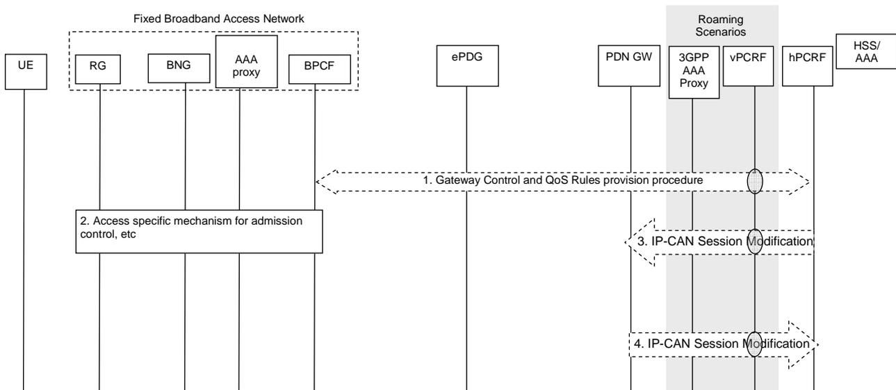
**Figure 8.3.7-1: Network-initiated dynamic policy control procedure in un-trusted BBF IP Access for DSMIPv6 on S2c**
