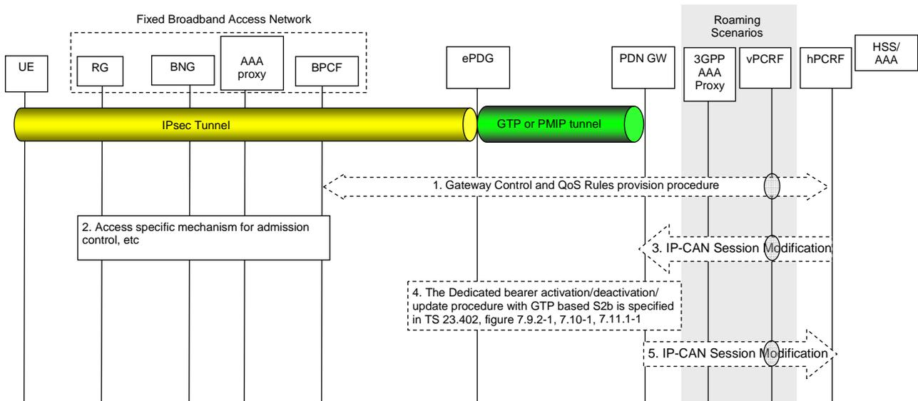
**Figure 7.6-1: Network-initiated dynamic policy control procedure**
