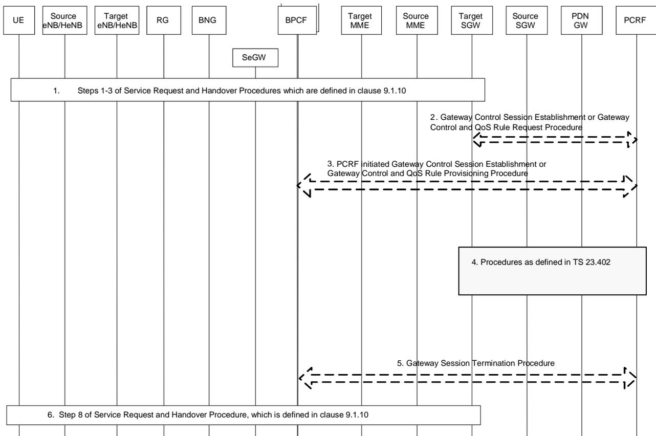
**Figure 9.2.8-1: Service Request and Handover Procedures-S5/S8 PMIP-based**
