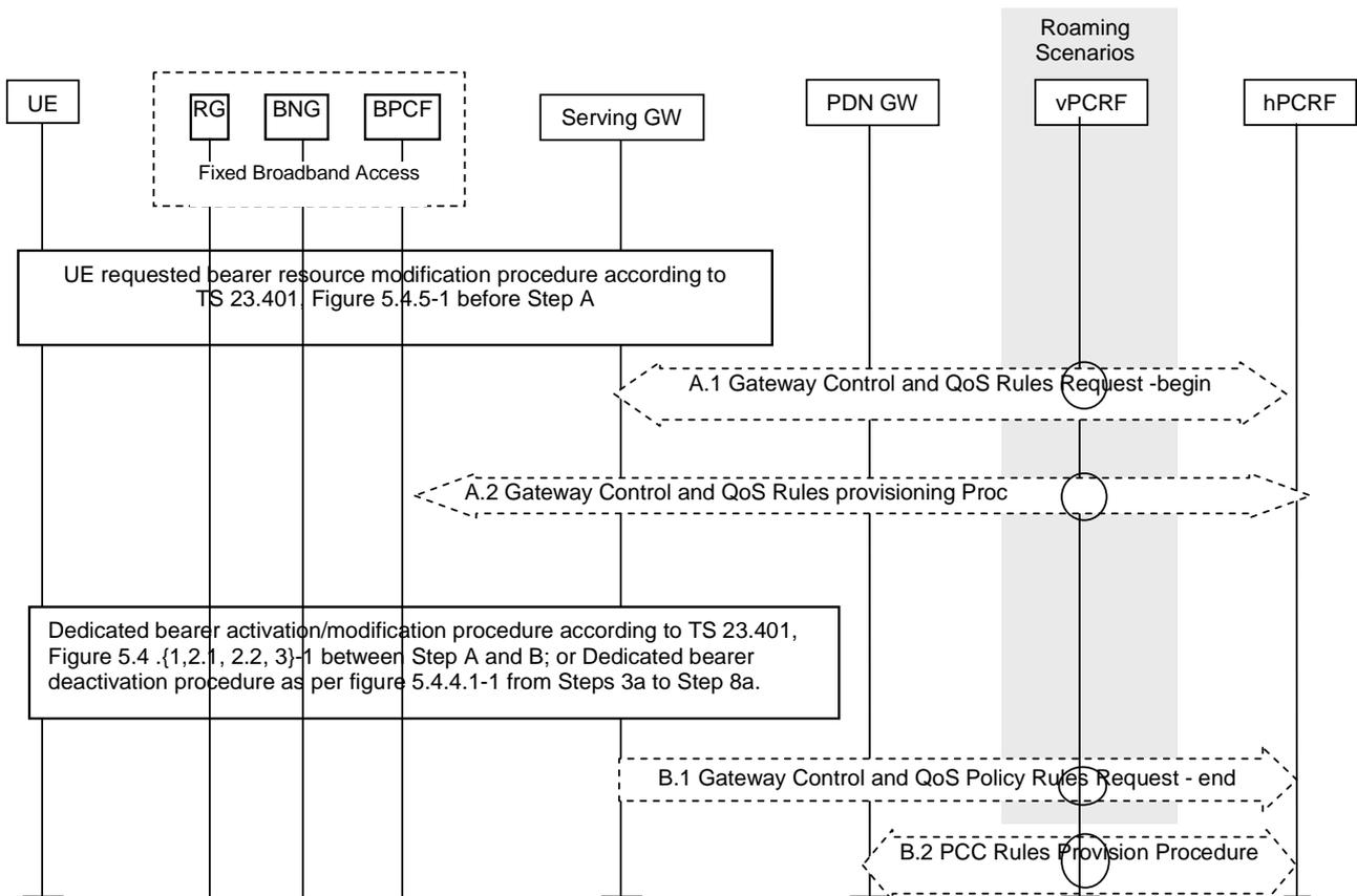
**Figure 9.2.6-1: UE-initiated resource request/release with PMIP-based S5/S8**
