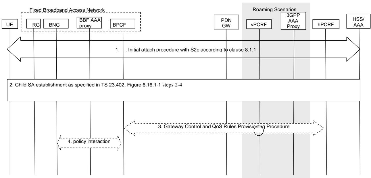
**Figure 8.2.10-1 Activation of enhanced security for S2c**
