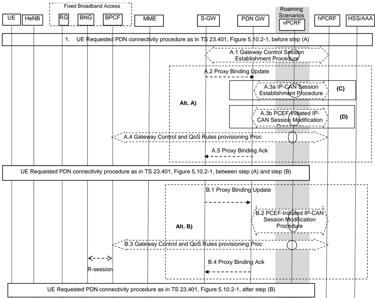
**Figure 9.2.7-1: UE requested PDN connectivity with PMIP-based S5 or S8**
