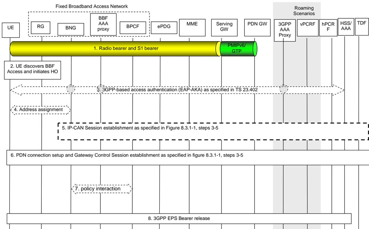
**Figure 8.3.5-1: E-UTRAN to untrusted Fixed Broadband Access Handover with DSMIPv6 on s2c**
