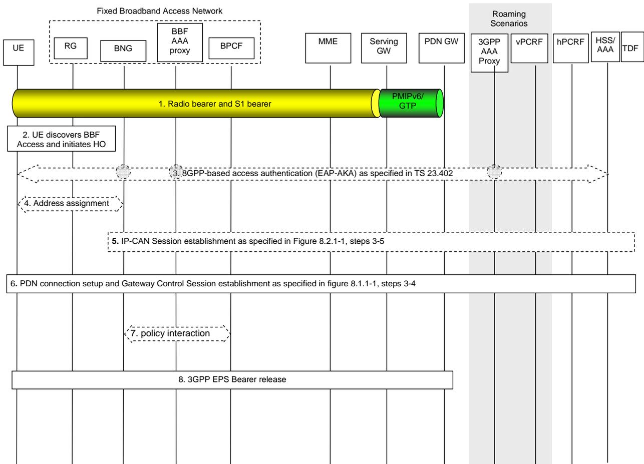
**Figure 8.2.5-1: E-UTRAN to Trusted Fixed Broadband Access Handover with DSMIPv6 on s2c**
