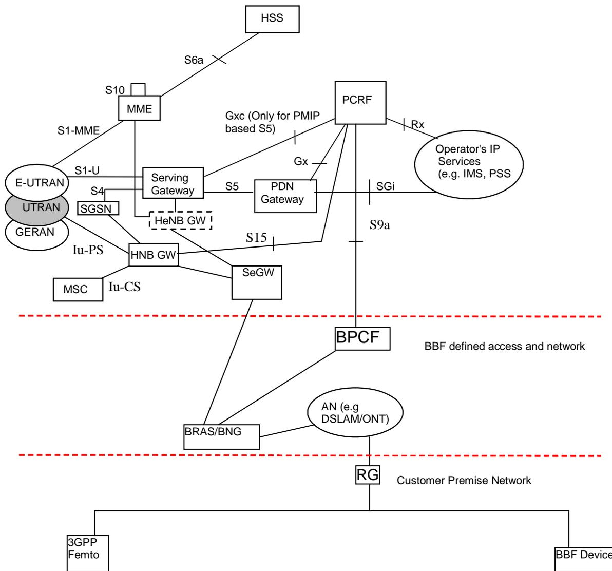
**Figure 4.3.2-1: Non-Roaming Architecture**
