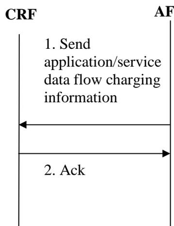
**Figure 7.0a: AF input to provision of charging rules**
