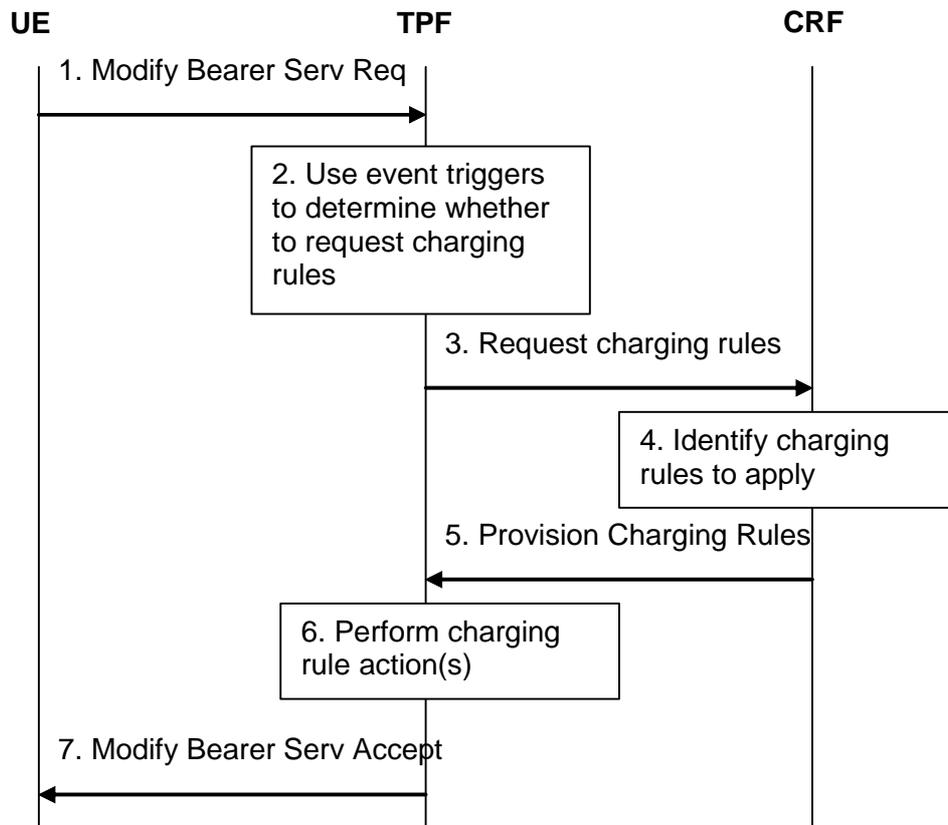
**Figure 7.2a: Bearer Service Modification triggered Charging Rule Request**
