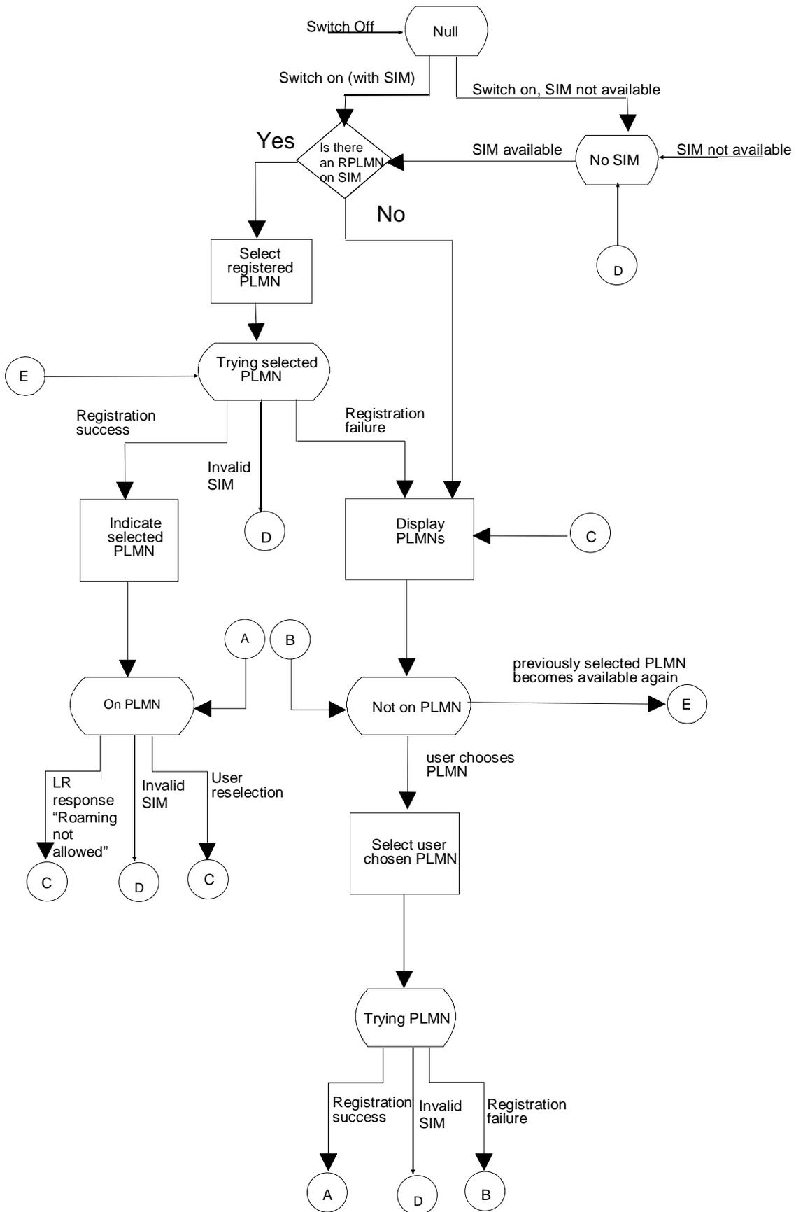
Figure 2b: PLMN Selection State diagram (manual mode)
