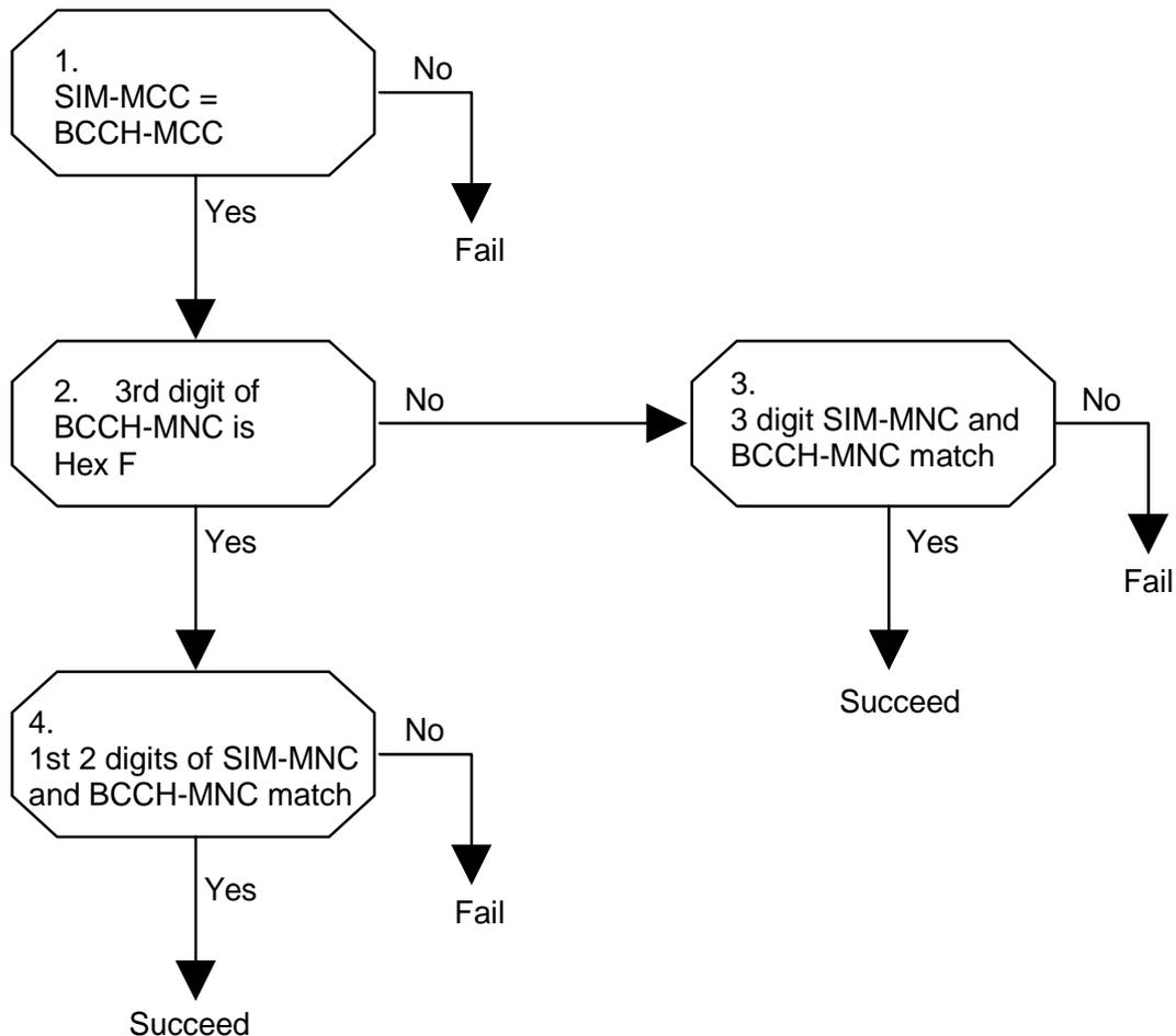
**Figure A.1: HPLMN Matching Criteria Logic Flow for mobiles which support GSM and DCS1800 (informative)**
