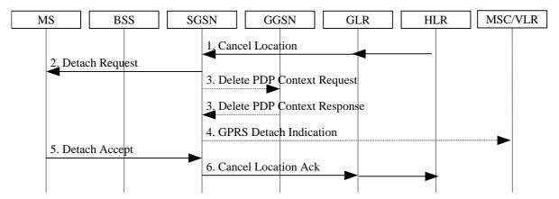
Figure 7.3/9: HLR-Initiated GPRS Detach Procedure
