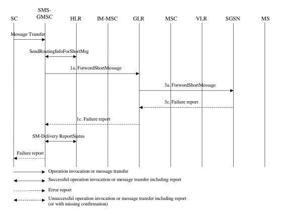
Figure 7.7/5d): Short message transfer attempt failing due to error at the SGSN
