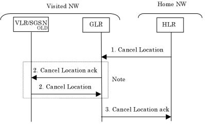
Note: This procedure is initiated only when the serving node doesn't support SC feature
