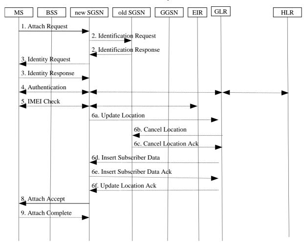
Figure 7.3/2: GPRS Attach Procedure involving GLR (new SGSN and old SGSN are under in the same GLR)
