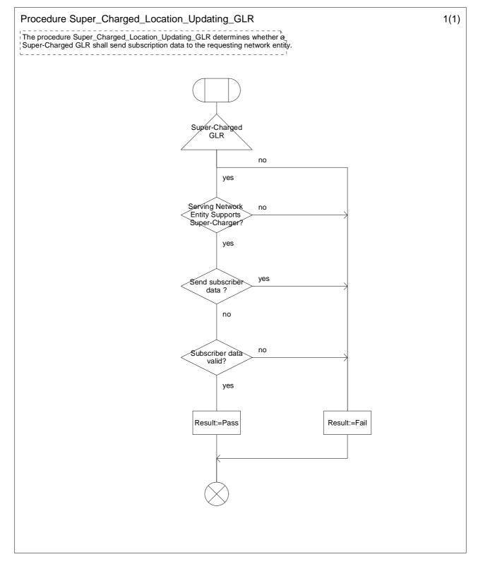
Figure 7.13/5: Procedure Super\_Charged\_Location\_Updating\_GLR
