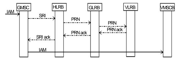
Figure 7.2/12: Information flow for retrieval of routeing information for a basic mobile terminated call
