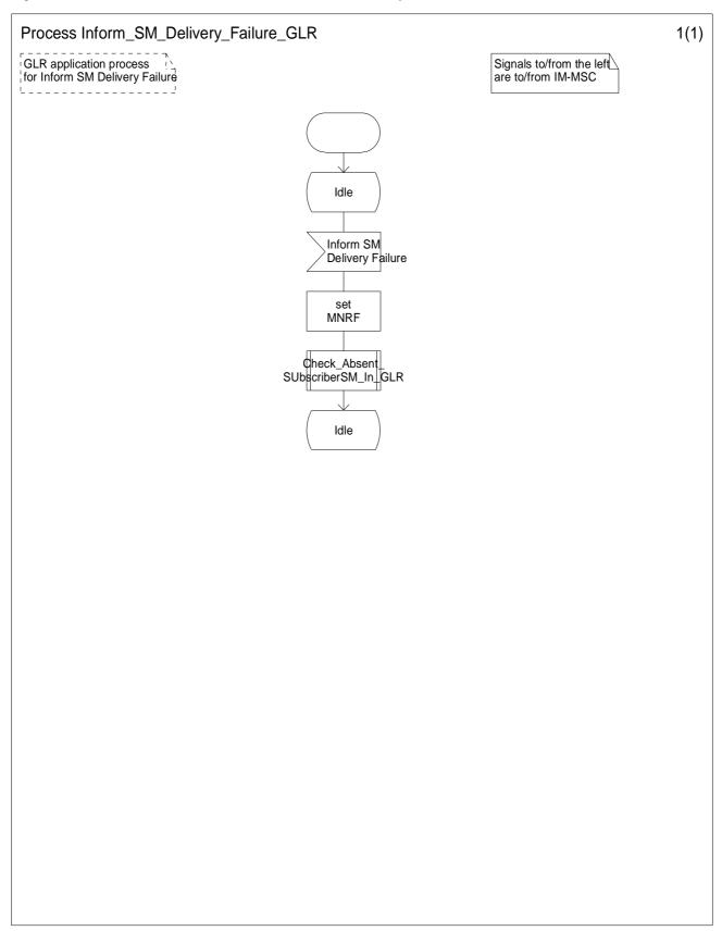
Figure 7.7/7: Process Inform\_SM\_Delivery\_Failure\_GLR
