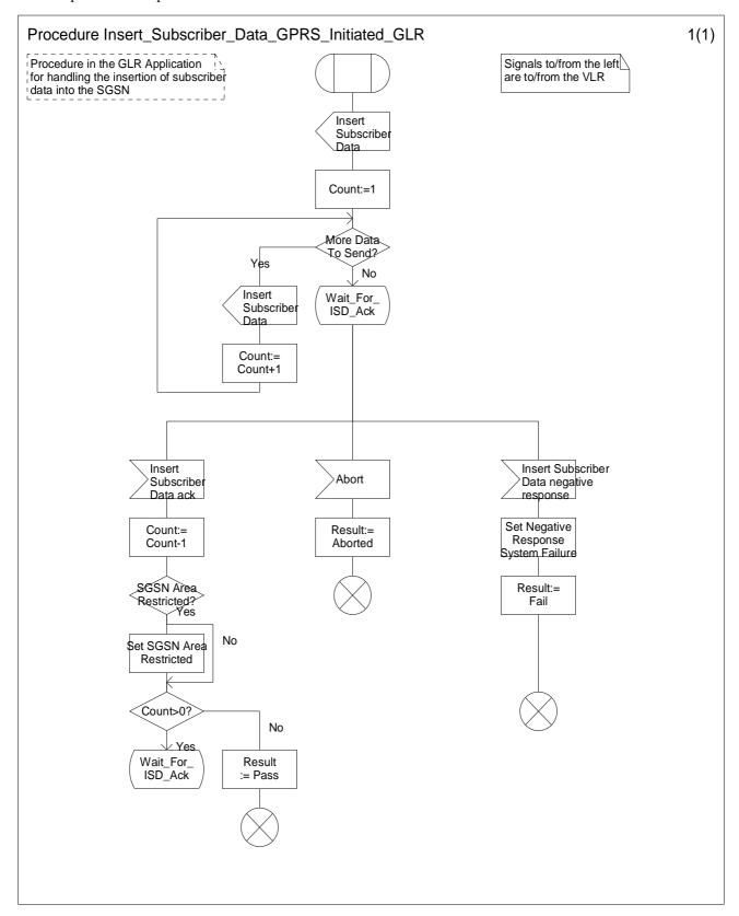
Figure 7.3/7: Procedure Insert\_Subscriber\_Data\_GPRS\_Initiated\_GLR
