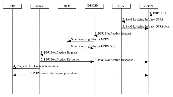
Figure 7.3/15: Successful Network-Requested PDP Context Activation Procedure
