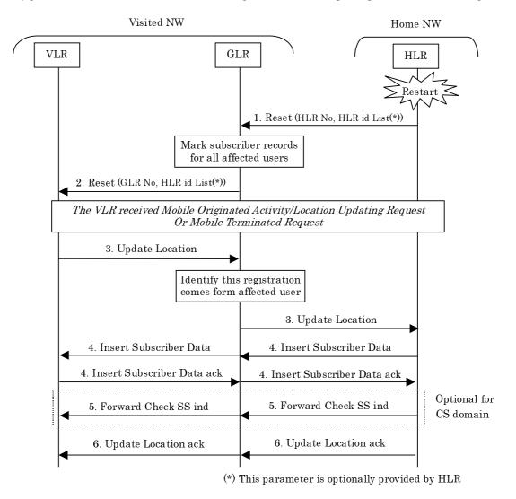
Figure 7.6/2: Recovery procedure of HLR Failure
