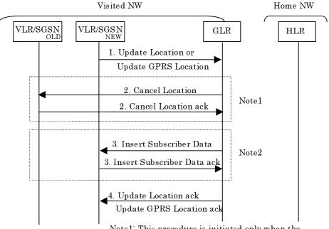
Note1: This procedure is initiated only when the serving node doesn't support SC feature
