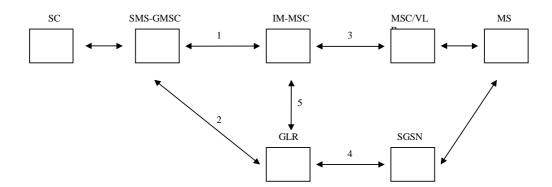
Figure 7.7/2: The main network structure serving as a basis for the SM MT with GLR
