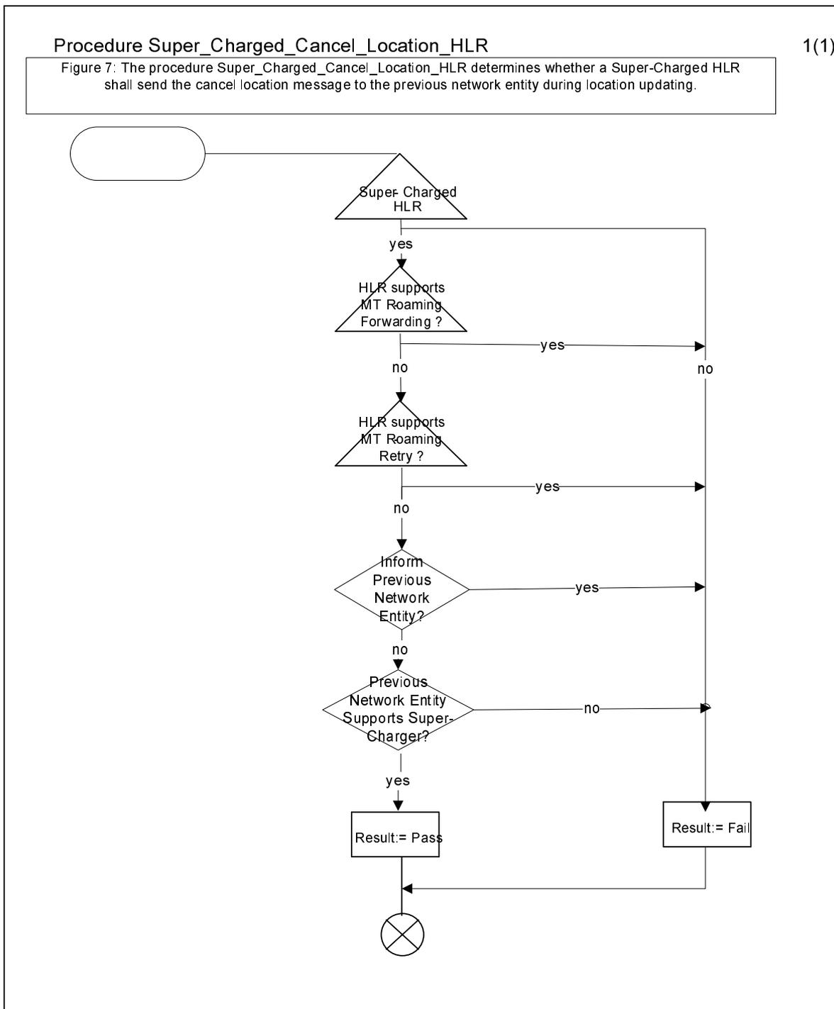
**Figure 7: Procedure Super\_Charged\_Cancel\_Location\_HLR**
