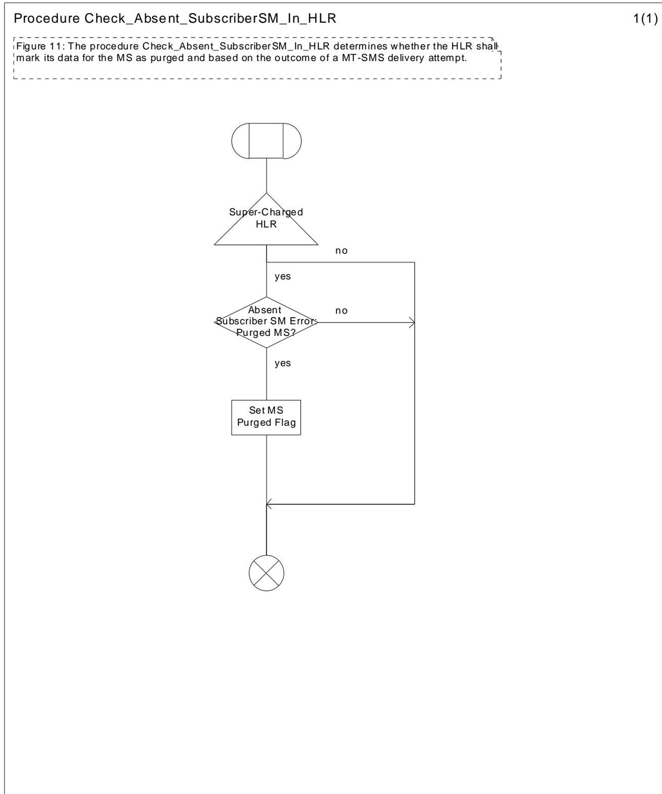
Figure 11: Procedure Check\_Absent\_SubscriberSM\_In\_HLR
