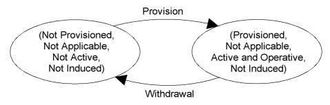
Figure 2.4: State transition model for AoCC
