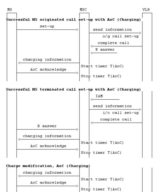
Figure 2.3 (sheet 2 of 2): Information flow for Advice of Charge (Charging)
