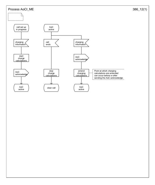
Figure 1.2: SDL diagram of advice of charge (information) in the mobile equipment
