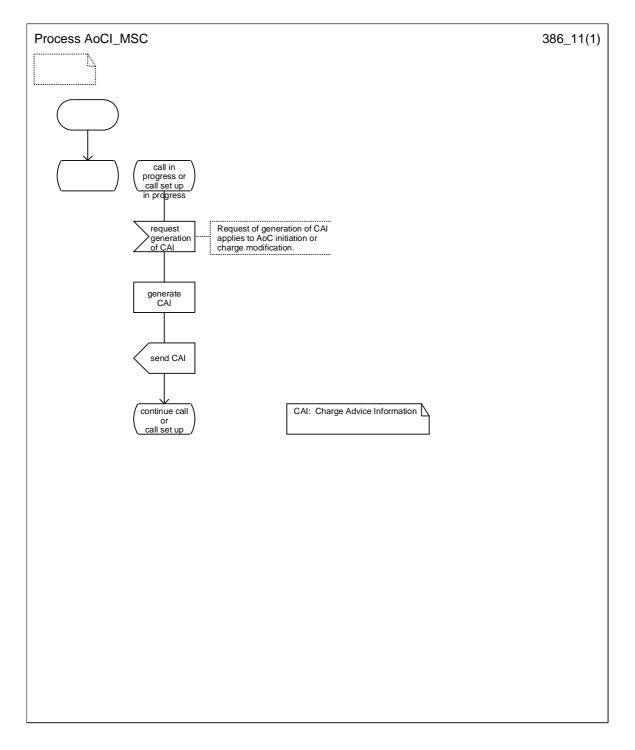
Figure 1.1: SDL diagram of advice of charge (information) in the MSC
