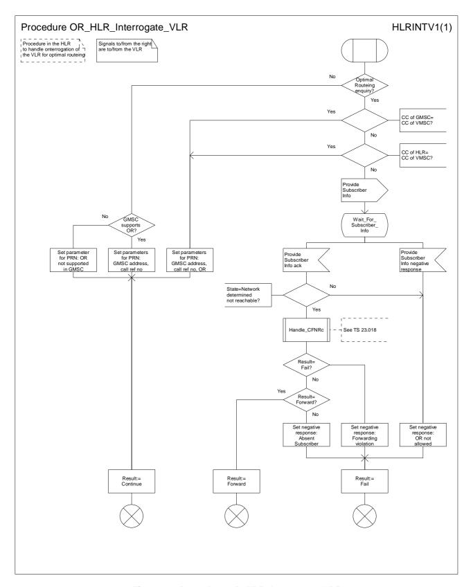
Figure 11: Procedure OR\_HLR\_Interrogate\_VLR
