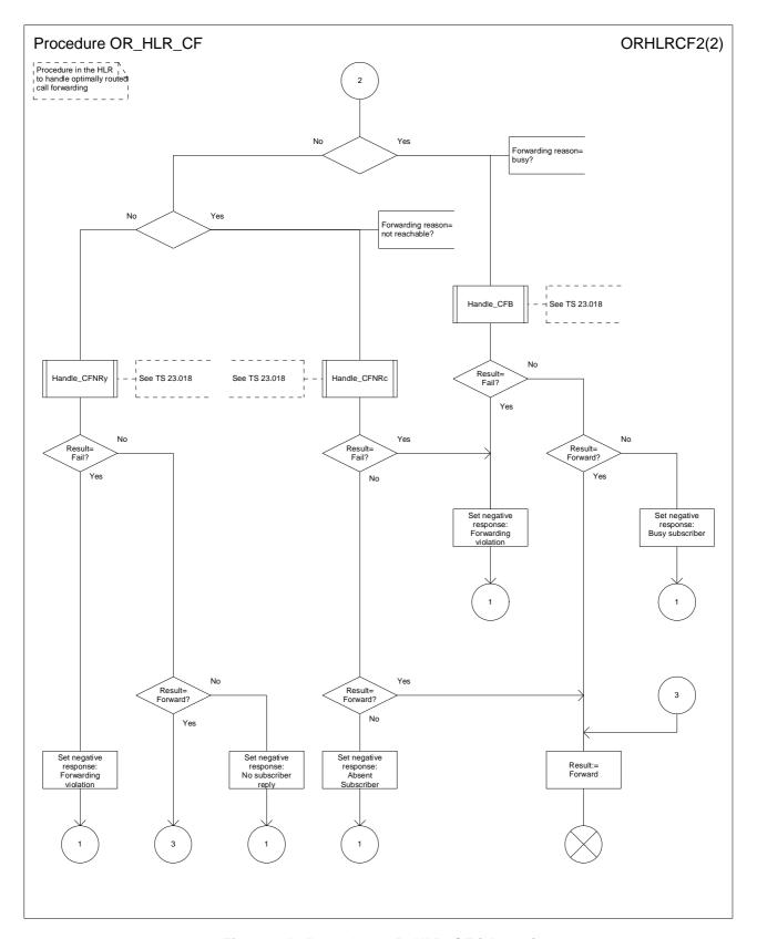
Figure 10b: Procedure OR\_HLR\_CF (sheet 2)
