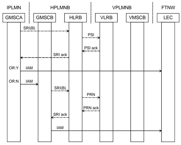
NOTE: HLRB may send a PRN to VLRB, and receive a PRN negative response indicating absent subscriber, to determine that CFNRc should be invoked.
