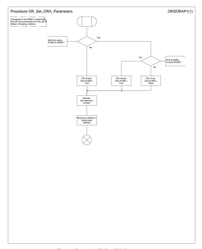
Figure 6: Procedure OR\_Set\_ORA\_Parameters
