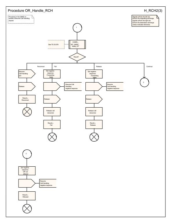
Figure 7b: Procedure OR\_Handle\_RCH (sheet 2)
