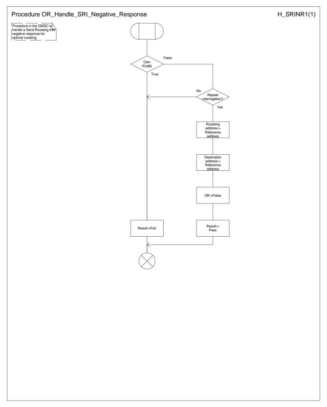
Figure 9: Procedure OR\_Handle\_SRI\_Negative\_Response
