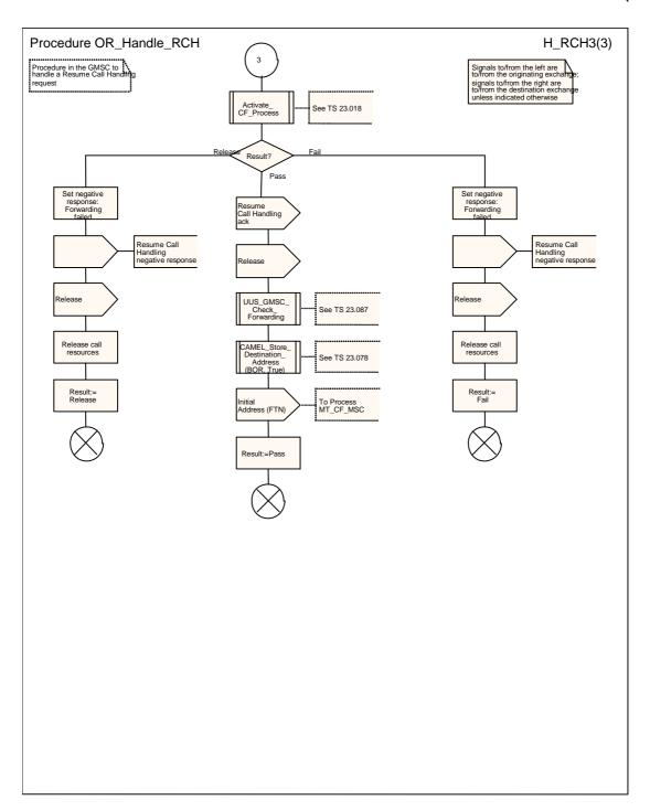
Figure 7c: Procedure OR\_Handle\_RCH (sheet 3)
