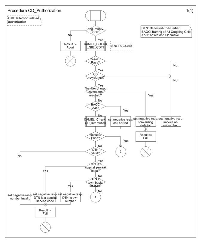
Figure 7.1 (sheet 1): Procedure CD\_Authorization
