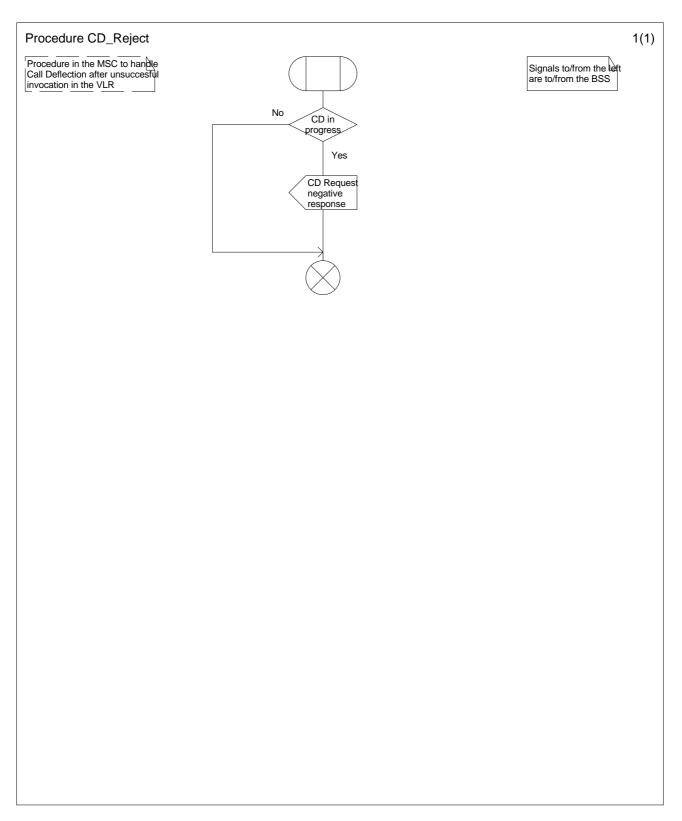
Figure 6.2: Procedure CD\_Reject
