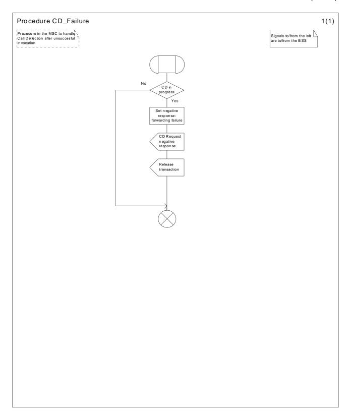
Figure 6.3: Procedure CD\_Failure
