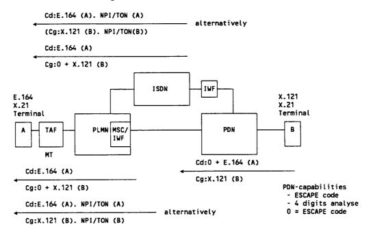
Figure 03.70/7: Interworking PDN-ISDN-PLMN (PDN 4 digits analysis)
