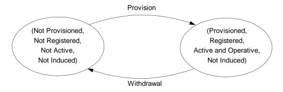
Figure 1: State transition model for eMLPP
