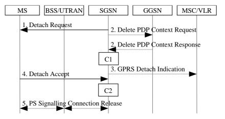
Figure 24: SGSN-Initiated GPRS Detach Procedure
