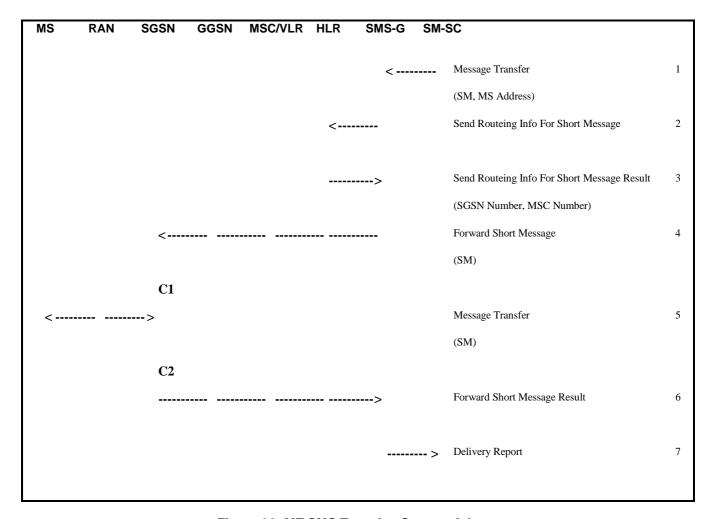
Figure 96: MT SMS Transfer, Successful
