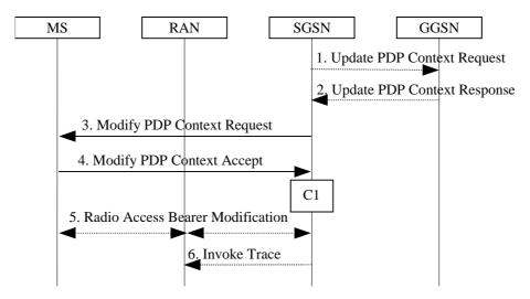
Figure 70: SGSN-Initiated PDP Context Modification Procedure
