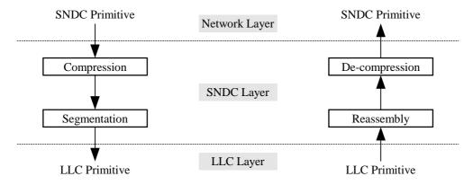
Figure 81: Sequential Invocation of SNDC Functionality
