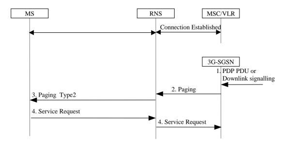
Figure 59: PS Paging With RRC Connection for CS
