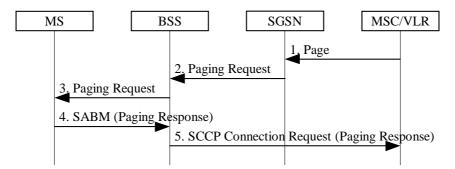
Figure 18: CS Paging Procedure in A/Gb mode
