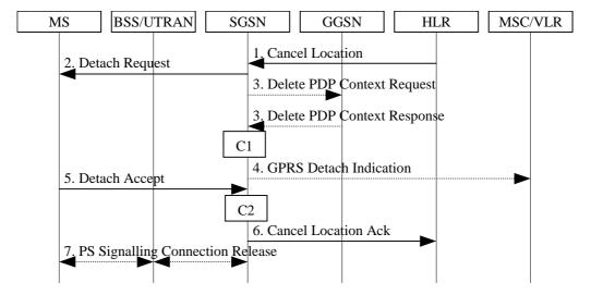
Figure 25: HLR-Initiated GPRS Detach Procedure
