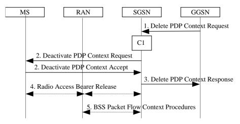
Figure 77: GGSN-initiated PDP Context Deactivation Procedure
