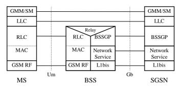
Figure 7: Control Plane MS - SGSN in A/Gb mode
