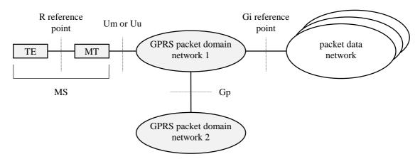
Figure 1: GPRS Access Interfaces and Reference Points
