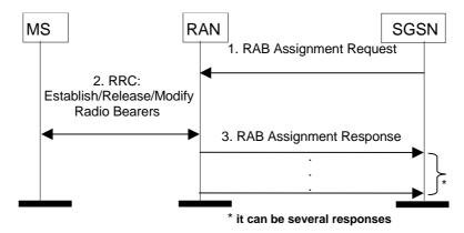
Figure 90: RAB Assignment Procedure
