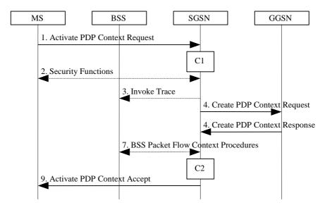
Figure 63: PDP Context Activation Procedure for A/Gb mode
