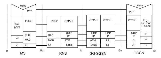
Figure 83: Iu mode User Plane for PDP Type PPP
