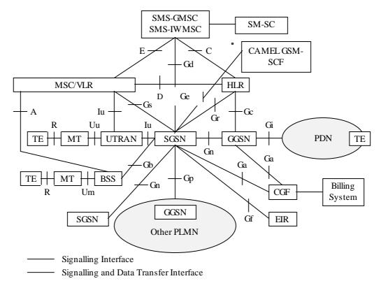
Figure 2: Overview of the GPRS Logical Architecture
