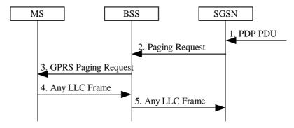
Figure 56: GPRS Paging Procedure
