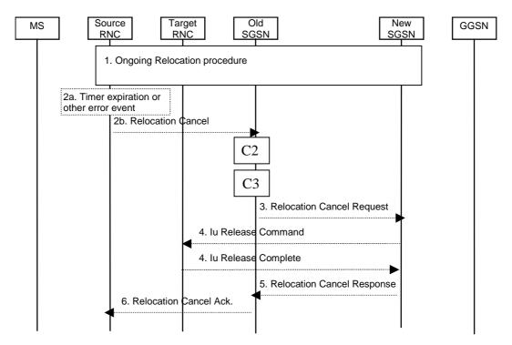
Figure 44: SRNS Cancel Relocation Procedure
