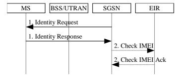
Figure 31: Identity Check Procedure
