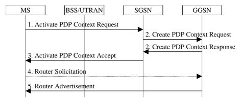
Figure 62: IPv6 Stateless Address Autoconfiguration Procedure
