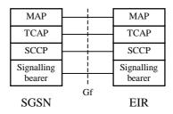
Figure 11: Control Plane SGSN - EIR
