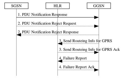
Figure 68: Protection Procedure
