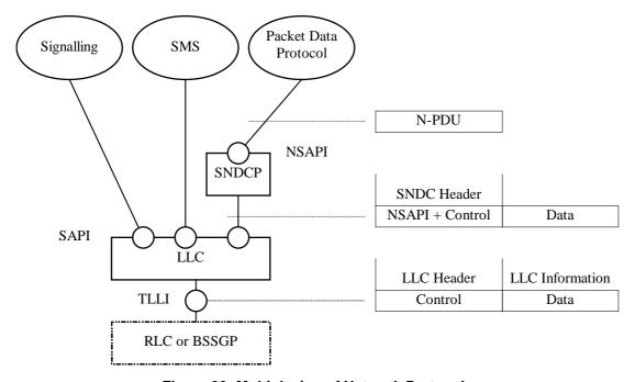
Figure 80: Multiplexing of Network Protocols
