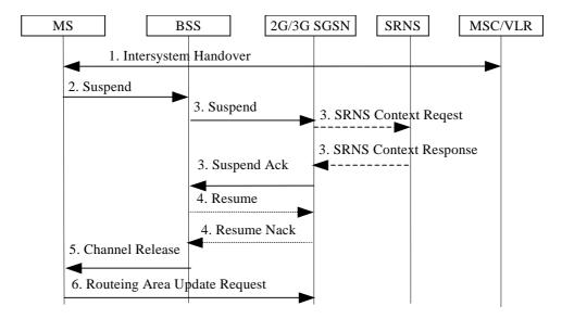
Figure 101: Suspend and Resume Procedure for intra-SGSN
