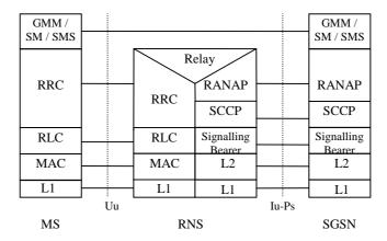
Figure 8: Control Plane MS - SGSN in lu mode
