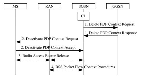
Figure 76: SGSN-initiated PDP Context Deactivation Procedure
