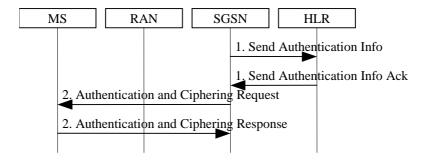
Figure 27: GSM Authentication Procedure
