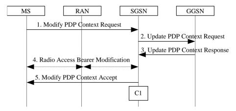
Figure 72: MS-Initiated PDP Context Modification Procedure
