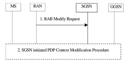
Figure 73: RAN-initiated RAB Modification Procedure
