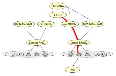
Figure 38: After SRNS Relocation and Routeing Area Update
