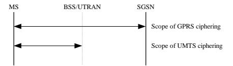
Figure 30: Scope of Ciphering
