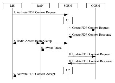
Figure 64: PDP Context Activation Procedure for Iu mode
