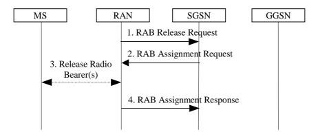
Figure 78: RAB Release Procedure
