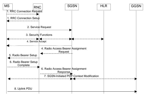
Figure 50: MS Initiated Service Request Procedure
