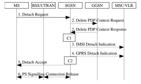
Figure 23: MS-Initiated Combined GPRS / IMSI Detach Procedure
