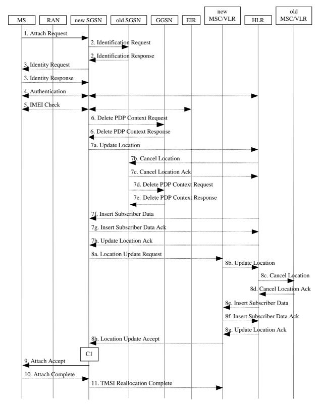
Figure 22: Combined GPRS / IMSI Attach Procedure
