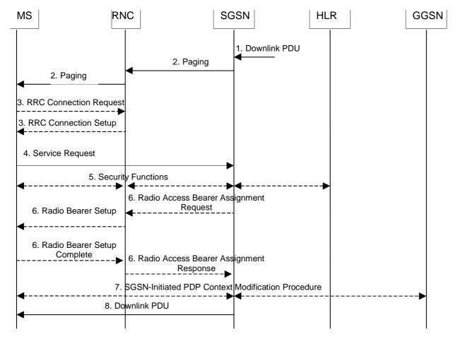
Figure 51: Network Initiated Service Request Procedure
