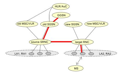
Figure 37: Before SRNS Relocation and Routeing Area Update
