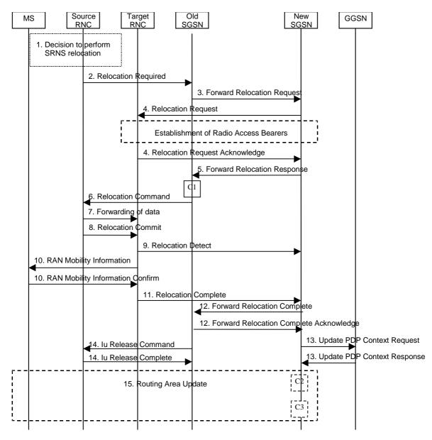
Figure 39: SRNS Relocation Procedure
