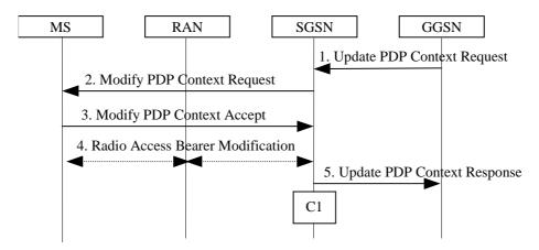
Figure 71: GGSN-Initiated PDP Context Modification Procedure
