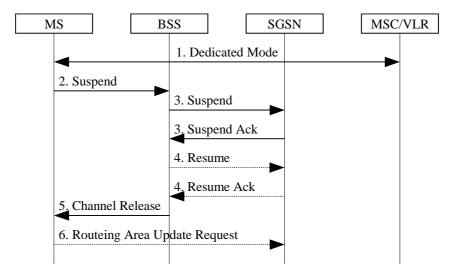
Figure 99: Suspend and Resume Procedure for intra SGSN
