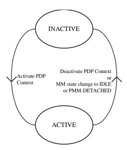
Figure 61: Functional PDP State Model
