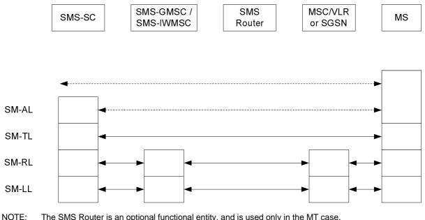
TE: The SMS Router is an optional functional entity, and is used only in the MT case. Figure 7: Protocol layer overview for the Short Message Service
