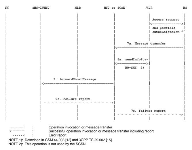
Figure 18d): Short message transfer attempt failing due to error at the SMS-IWMSC
