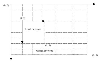
In Compact Coordinate System, coordinates are restricted to certain positions which are the cross points of a grid. The grid is defined in the WVG data header, set by a group of parameters. The grid lines along with x axis or y axis may be unevenly distributed.
