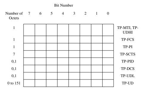
Bits 7 and 5 - 2 in octet 1 are presently unused and the sender shall set them to zero. If any of these bits is non-zero, the receiver shall not examine the other field and shall treat the TP-Failure-Cause as "Unspecified error cause".
