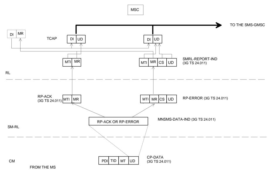
NOTE: The cause carried via UD of TCAP is not the cause supplied via RP-ERROR but is the cause resulting from application of the mapping specified by table 8.5 of 24.011[13].
