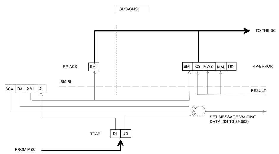
NOTE 1: The MAP operation "SetMessageWaitingData" is invoked only if a cause "Absent Subscriber" is carried in TCAP UD. NOTE 2: The cause delivered to the SC is not necessarily the cause carried via TCAP but is one of the set specified by table 03.40/1.
