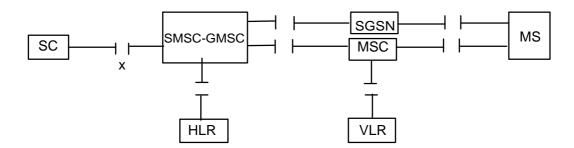
NOTE: Since the short message mobile terminated procedure covers the functionality required at SM-RL for transferring TPDUs from SC to MS, the procedure described covers both short message (SMS-DELIVER) and status report (SMS-STATUS-REPORT) transfer. The term "short message transfer" therefore, in this clause, covers both cases.
