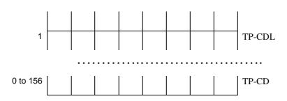
NOTE: The maximum guaranteed length of TP-CD is 146 octets. In order to achieve the maximum stated above (156 octets), the TP-DA field must have a length of 2 octets.
