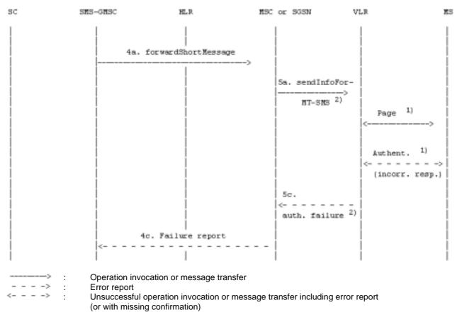
NOTE 1): Described in GSM 04.08 [12] and 3GPP TS 29.002 [15]. If the SGSN is used, Paging and Authentication are performed from SGSN. NOTE 2): This operation is not used by the SGSN.
