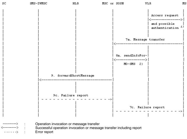
NOTE 1): Described in GSM 04.08 [12] and 3GPP TS 29.002 [15]. NOTE 2): This operation is not used by the SGSN.
